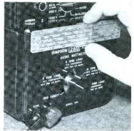
Fig. 9. Slide-rule device used on three of the new Simpson Add-A-Testers.
