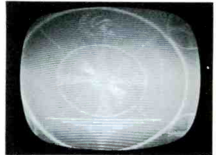
Fig. 3. Negative picture indicates extreme overloading of video circuits.
