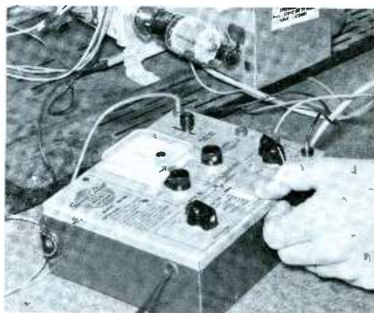
Fig. 4. Sencore SS105 isolates sweep trouble to oscillator, output or yoke.
