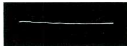
Fig. 6. Fault in either oscillator or output stage could cause no sweep.
