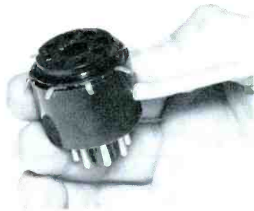
Fig. 5. Special tube socket adapter of Model SS105 for in-circuit testing.
