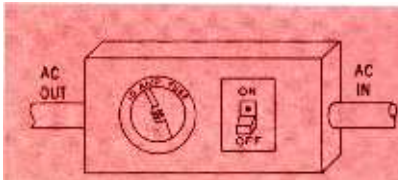
Fig. 2. Individual on-off switches and fuses for each bench are desirable.
