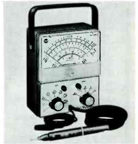
Fig. 1 RCA VoltOhmyst, Model WV-500A, solid-state electronic VOM.
