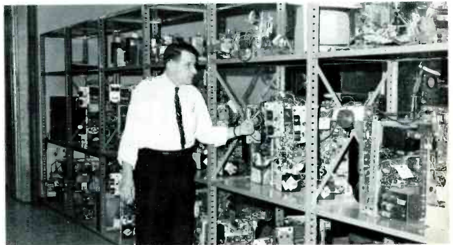
THE BRANCH MANAGER, W. A. Sharp, inspects repaired sets in the 'out' rack, which forms a wall of the service area. Inside technicians place the chassis in this rack when tagged and completed. The racks are open on both sides, making it easier for the sets to be stored by the benchmen on the one side, and picked up on the other side by the outside man on his way to the service truck.
