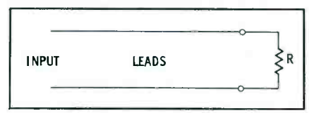
Fig. 5. If R has proper value, it makes no difference how long the leads are.
