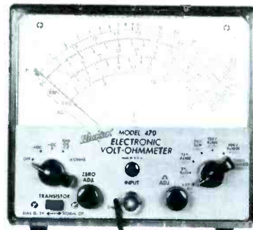
Fig. 5. Meter face of new VTVM extends over almost entire width of case.
