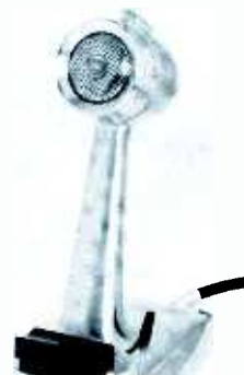
Turner Model 250—dynamic Frequency response: 100-10,000 cps Output level: -54 db Impedance: high Pickup pattern: omnidirectional
