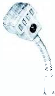
Reslo "Avon"—ribbon Frequency response: 20-15,000 cps Output level: -58 db Impedance: low, medium, or high Pickup pattern: super-cardioid
