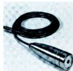
Ronette "Ronomike"—crystal Frequency response: 30-10,000 cps Output level: -55.4 db Impedance: high Pickup pattern: semidirectional
