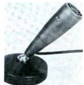
RCA Model BK-1A—dynamic Frequency response: 60-10,000 cps Output level: -52 db Impedance: 30, 150, or 250 ohms Pickup: non- or semidirectional
