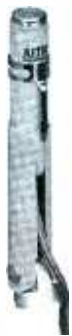
Atec Model M20—condenser Frequency response: 20-15,000 cps Output level: -59, -53, -49, -44 db Impedance: 30/150/600/10K ohms Pickup pattern: omnidirectional
