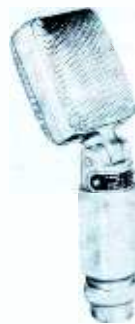
Reslo "Symphony"—ribbon Frequency response: 18-15,000 cps Output level: -58 db Impedance: low, medium, or high Pickup pattern: bidirectional
