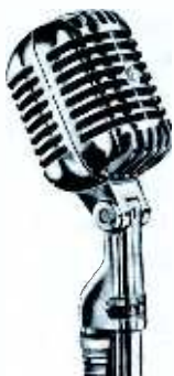
Shure Model 55S—dynamic Frequency response: 50-15,000 cps Output level: -54, -55, -57 db Impedance: 30-50/150-250/35K Pickup pattern: ultra-cardioid
