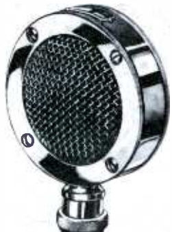
Astatic Model D-104—ceramic Frequency response: 30-7,500 cps Output level: -47 db Impedance: high Pickup pattern: cardioid
