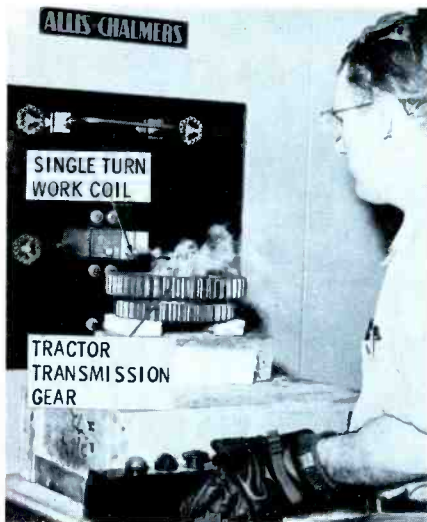
Fig. 6. Heat is used to anneal gears to make them tough and wear-resistant.
