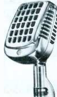
Shure Model 737A—crystal Frequency response: 60-10,000 cps Output level: -53 db Output impedance: high Pickup pattern: cardioid
