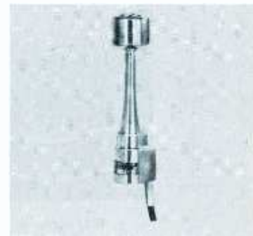
Turner Model 80—crystal Frequency response: 80-7,000 cps Output level: -54 db Output impedance: 25,000 ohms Pickup pattern: nondirectional
