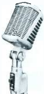
Astatic Model 77—dynamic Frequency response: 30-15,000 cps Output level: -52 db Output impedance: 30-50, 150-250, 40K Pickup pattern: cardioid
