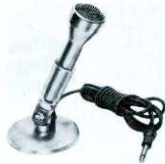
Sonotone Model CM-10—ceramic Frequency response: 50-13,000 cps Output level: -62 db Output impedance: high Pickup pattern: omnidirectional
