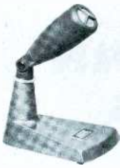
Altec-Lansing 661—dynamic Frequency response: 30-15,000 cps Output level: -55 db Output impedance: 30-50, 150-250, 20K Pickup pattern: omnidirectional
