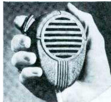
Shure Model 101C—carbon Frequency response: 300-4,000 cps Output level: 5 db below 1v @ 100 mb Output impedance: 50-100 ohms Pickup pattern: semidirectional
