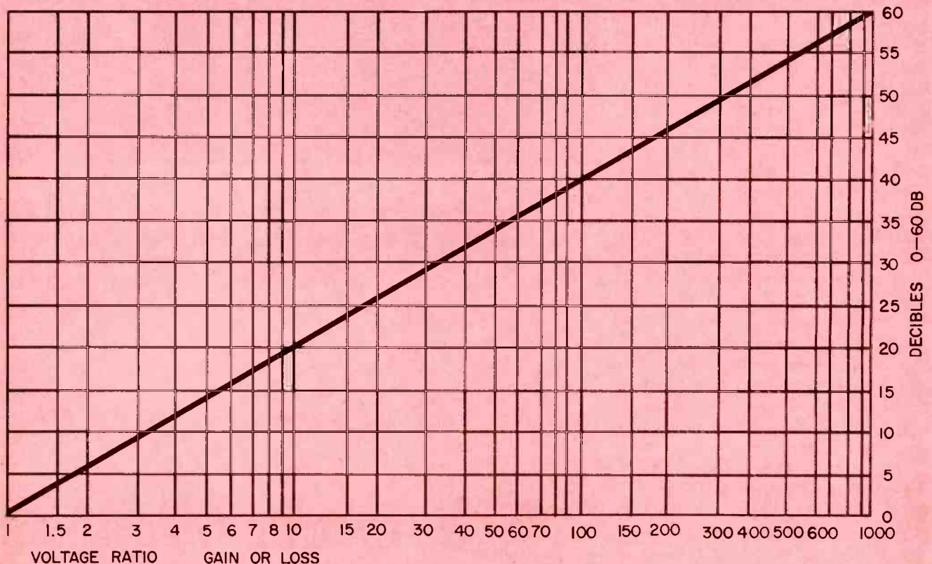
Graph for converting voltage-ratio figures to db equivalents.
