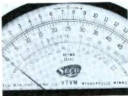
Fig. 6. A special ohms scale is provided on Seco meter for standard values.
