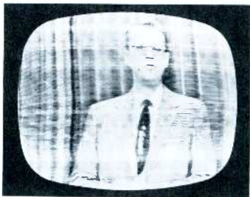
B. Streaks are due to a broken wire in the antenna lead or to a loose terminal connection.
