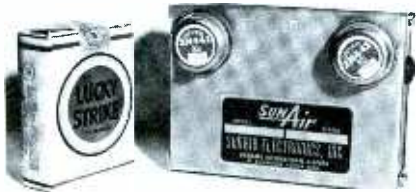
Fig. 6. Complete transistorized DC-to-DC converter fits into a small package.
