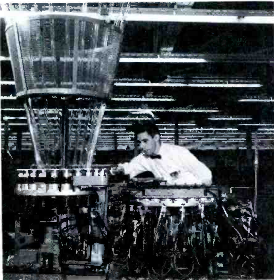
The new double-turret sealax is an important new development. Oil-diffusion pumps work in series with mechanical pumps to produce the most nearly perfect vacuum possible.
