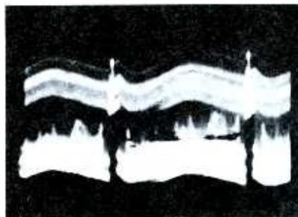
Fig. 6. Plate waveform of V1 with 60-cycle modulation (Scope sweep 30 cps).
