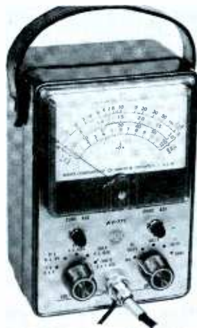
Fig. 4. RCA's new Junior VoltOhmyst incorporates meter burn-out protection.
