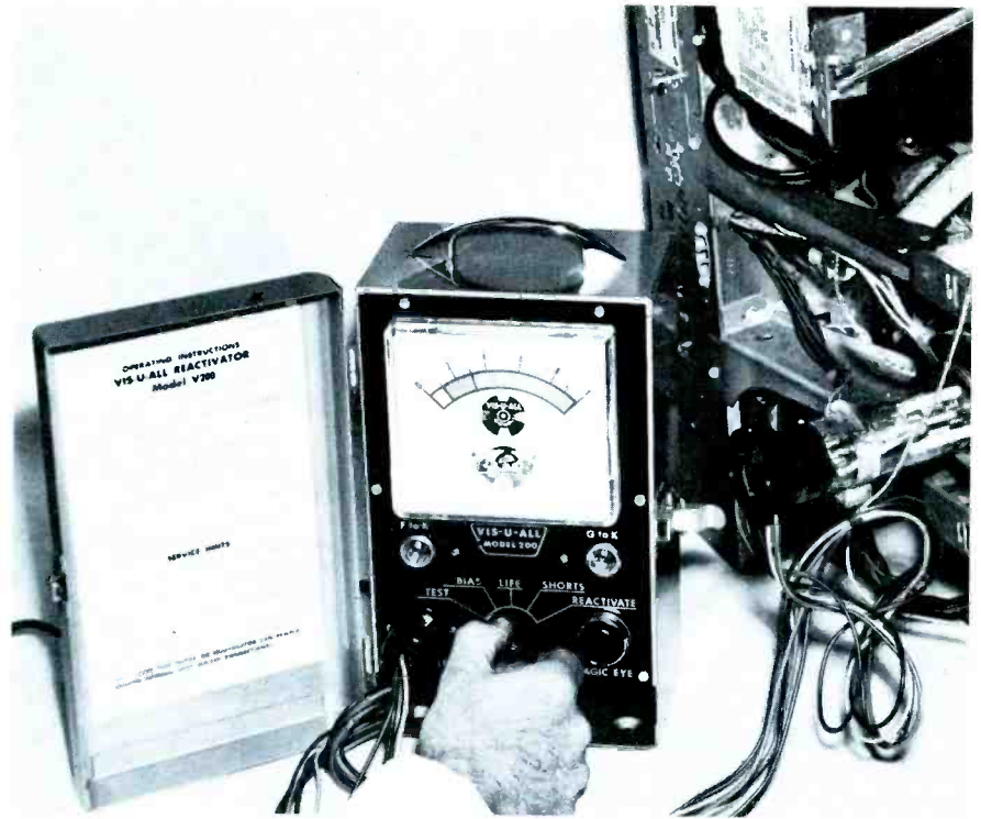
Fig. 7. Vis-U-All 200 performs four tests and reactivates picture tubes.
