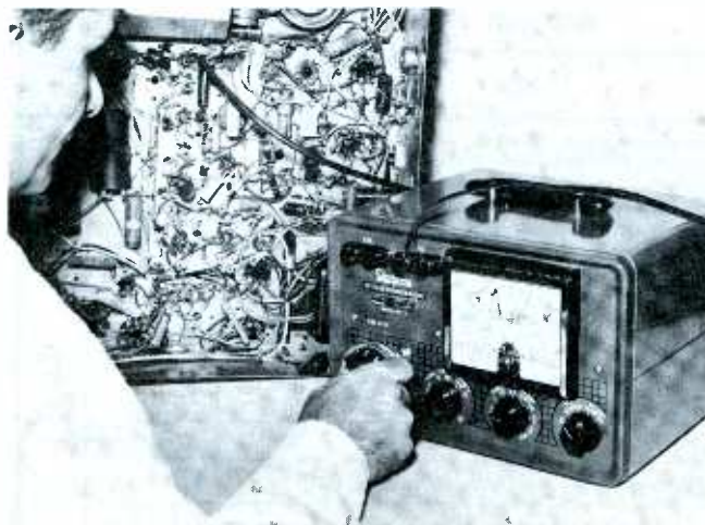
Fig. 1. Simpson's new 498-A field strength meter can be substituted for the tuner used in any television receiver.
