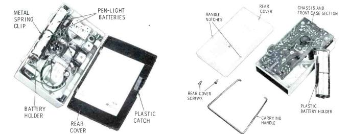
Fig. 2. In the Philco Model T-4, the case can be opened by prying out on clip and separating the two individual sections.
