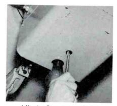
Adjusting Perma-Power Clutch
