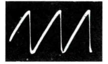
(B) Feedback sawtooth.Fig. 2. Waveforms in AFC grid circuit.
