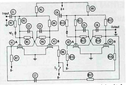
Fig. 3. Positive feedback from 2nd Eccles-Jordan reduces scale from 4 to 3.
