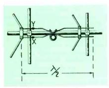
Fig. 18. Two-conductor coupling between T-matched sections. Lead-in goes to X-Y.
