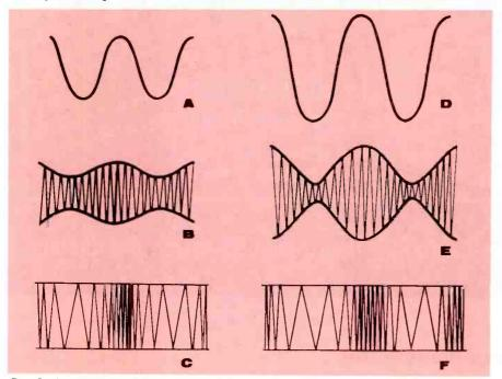
Fig. 1. Amplitude and frequency modulation of an RF carrier by 1-kc audio signals of two different strengths.
