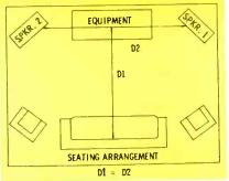
Fig. 7. Example of speaker placement with respect to listening area for stereo.
