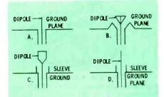
Fig. 2. "Sleeve-dipole" principle developed from whip-and-ground-plane array.
