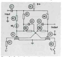
Fig. 1. Eccles-Jordan will change conduction status with each negative pulse.
