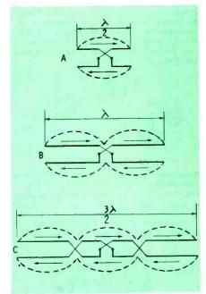
Fig. 4. Steps used in developing broadband response for Trio's wing dipole.
