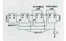
Fig. 5. Scale of 5 coupled to scale of 2 makes circuit into a decade counter.
