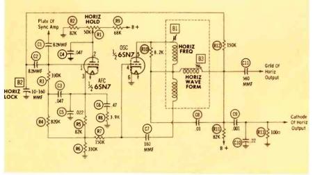
Fig. 1. Schematic of popular pulse-width AFC and oscillator circuit.
