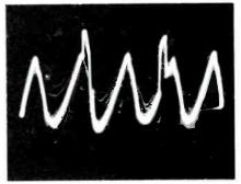
(B) AFC grid waveform.Fig. 4. Horizontal oscillator operating at about 25 kc produces these symptoms.
