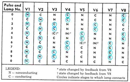
Fig. 7. Chart showing lamp connections and conditions under which each lights.
