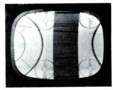
Fig. 3. This out-of-phase condition is due to improper horizontal AFC control.
