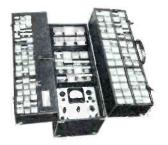
A caddy with built-in tube tester is being marketed by Vis-U-All Products Co., Grand Rapids, Mich. The tester provides checks for quality, grid-cathode or heater-cathode shorts, interelectrode leakage, grid emission, and gas. Sensitivity of the leak-
