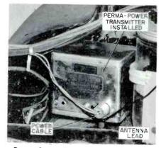
Perma-Power Transmitter Installation
