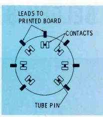
Fig. 5. Details of printed-board type tube socket that caused noisy operation.
