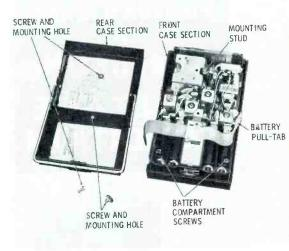
Fig. 4. Zenith portable incorporates a pull-out tape for quick removal of the battery cells.
