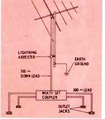
Fig. 1. Shop antenna system for strong signal areas where noise level is low. minimized. The down lead from the booster should be 72-ohm coaxial line to prevent noise pickup, and to simplify the job of providing multiple outlets in the shop. Suitable booster amplifiers, tap-off units and 72- to 300-ohm matching units that can be used to assemble the system shown in Fig. 2 are readily available through most electronic parts distributors.
