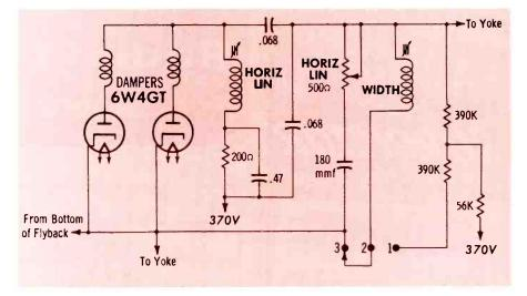
insufficient width. I have tried replacing the yoke, horizontal output transformer, linearity coil, and every capacitor between the horizontal oscillator and output stages. By the way, B+ voltage is normal.
