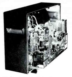
Fig. 1. In new General Electric "Designer" series, most of chassis is exposed when curved back cover is removed.
