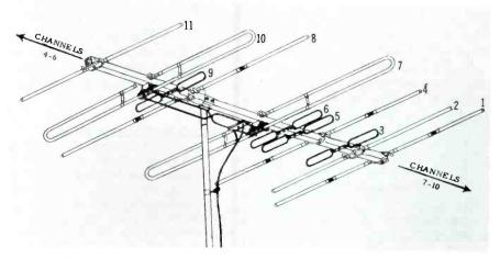
Fig. 13. Finney TCR-1 array receives selected signals from opposite directions.
