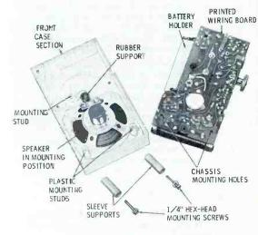
Fig. 6. Westinghouse H-655P5 chassis removed from the front section of its plastic case.
