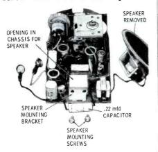
Fig. 8. Speaker of Silvertone 9202 must be removed to make parts accessible.
