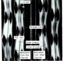
Fig. 3. Photomicrograph of stereo grooves cut with single modulation frequency. (Courtesy of Westrex Corp.)
