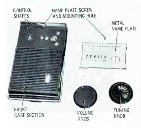
Fig. 5. To remove the chassis of the Royal "300," disassemble the name plate and control knobs.
