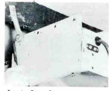
Securing Perma-Power Motor to Beam
