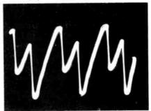
(B) Oscillator plate waveform.Fig. 5. Severe foldover such as this can be caused by improper AFC operation.
