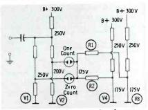
Fig. 6. Method of connecting lamps so they light for only one set of conditions.
