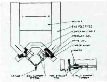
Fig. 2. Basic recording head showing coil placement and attachment to stylus.
