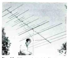
Fig. 15. Winegard Model CL-4X uses extra parasitic elements for added gain.
