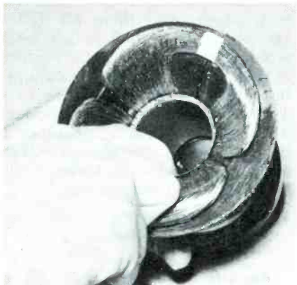
(C) Cement, position, and allow to dry.
