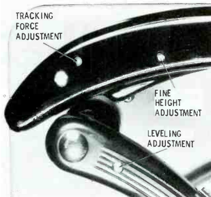
Fig. 8. Tone arm and stabilizer bar adjustments of Collaro "Conquest" changer.
