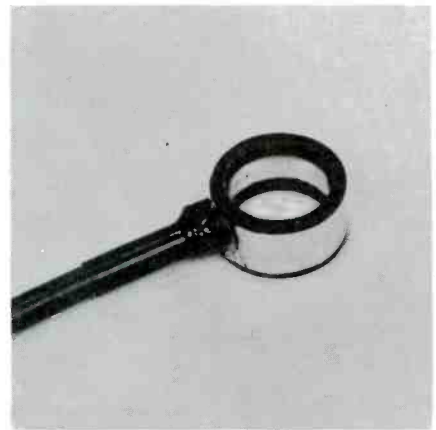
Fig. 3. Model 850 uses pickup rings to sample the signal from the receiver.
