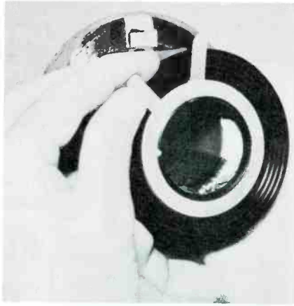
Fig. 6. Yoke cover with centering device not standard on most replacement units.
