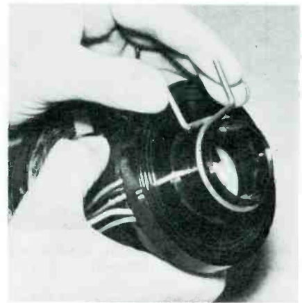
Fig. 7. Cover with clamping device holds deflection yoke in position.
