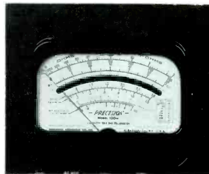
Fig. 4. Close-up of 120M meter shows mirrored scale which eliminates parallax.
