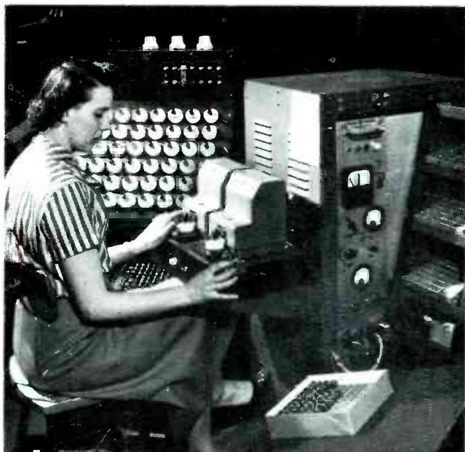
5 —Testing the tester. As a constant check on the accuracy of the automatic tester—samples from each lot tested, are retested on similar equipment used as a standard. Records are kept of all tests serving as data to feed back to design, manufacturing, and quality-control groups.
