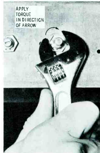
Fig. 5. Using adjustable wrench correctly.
