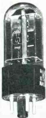
Fig. 2. Flakes in damper tube produced by arcing between cathode and filament.
