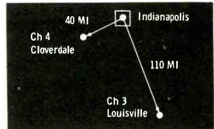
Fig. 8. Adjacent-channel interference is often encountered between these two stations in the Indianapolis area.
