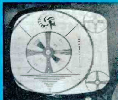
Fig. 8. Phasing ghost accompanied by slight picture shift.
