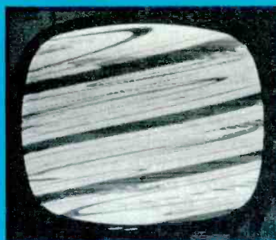
Fig. 4. Diagonal bars indicating loss of horizontal synchronization.
