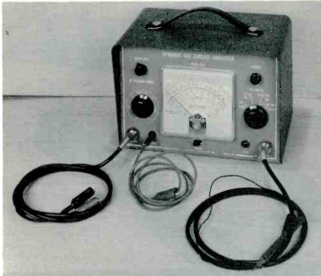
Fig. 1. Win-Tronix Model 825 Dynamic AGC Circuit Analyzer. The unit cuts time in servicing AGC systems.
