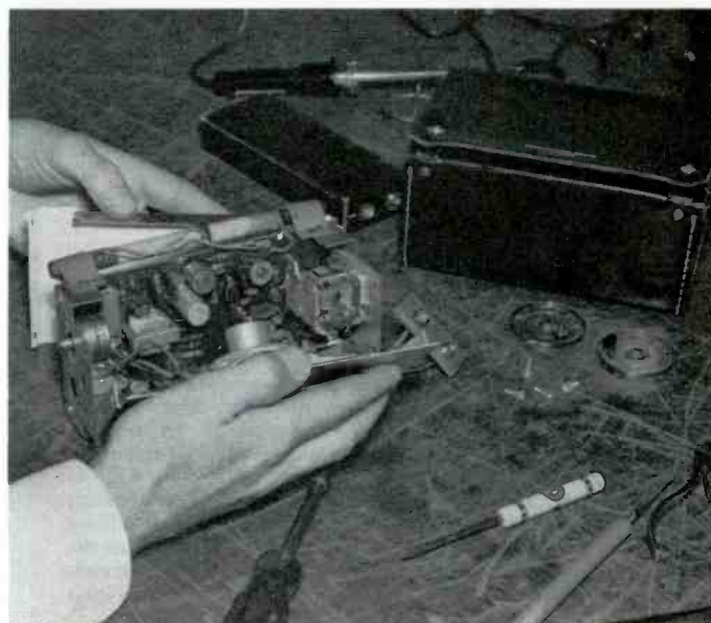
Fig. 2. Accessibility to test points on this Regency Model TR-6 is achieved by removing speaker panel and protective shield.
