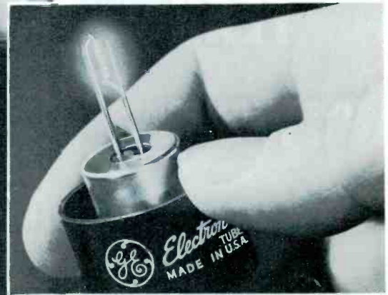
ABOVE: Tungsten "lightning rod" in G-E high-voltage rectifier tubes shields the filament from electrostatic pull of high anode voltages. Shorts, broken filaments are sharply reduced.
