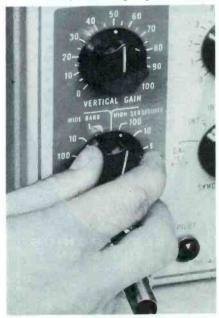
Fig. 1. Wide-Band—High-Sensitivity switch on an oscilloscope.
