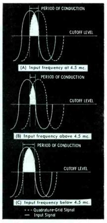
Fig. 3. Plate-current conduction in a quadrature-grid detector.
