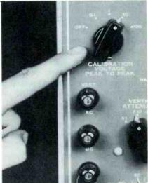
Fig. 4. Oscilloscope with an internal, switch-controlled calibrating voltage.
