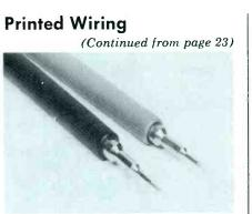
Fig. 3. Needle-pointed test leads.
