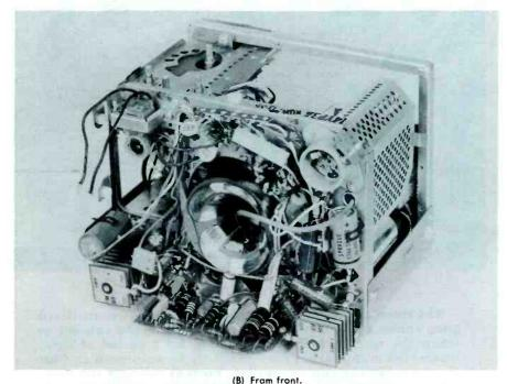
Fig. 3. Views of Admiral portable TV chassis.
