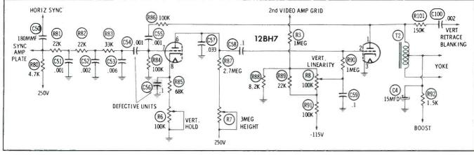
Fig. 3. RC-coupled vertical multivibrator.
