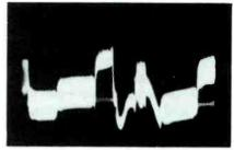
pe. (B) On a narraw-band scope. Fig. 2. Composite color signal.
