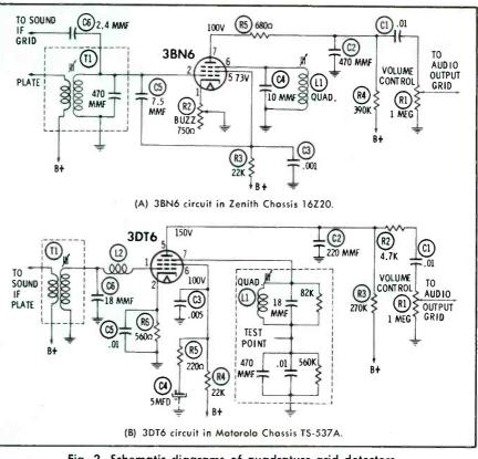
Fig. 2. Schematic diagrams of quadrature-grid detectors.
