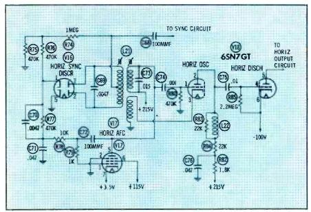
Fig. 1. Circuit diagram of the horizontal-sync stages in George's "tough dog" set.
