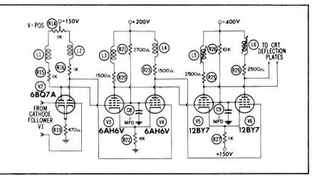
Fig. 3. In This Vertical System, Two Frequency-Governing Adjustments Are Used. These Are L5 and L6.
