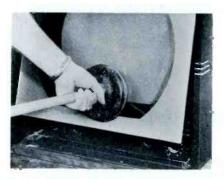
Fig. 1. Plunger Being Used to Remove Safety Glass from TV Set.
