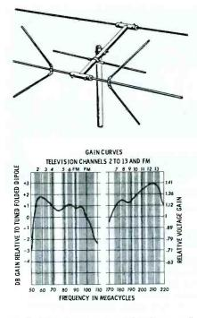
Fig. 2. Mallet Antenna With Wings and High-Frequency Reflector.
