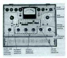
Fig. 6. Commercial Example of a Transconductance Tube Tester.
