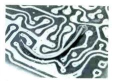
Fig. 4. Conductor Replaced With Wire.
