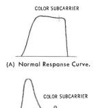
(B) Severe Attenuation of the Color Subcarrier Due to Multipath Reception.
