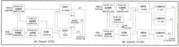
Fig. 6. Block Diagrams of Chrominance Sections of RCA Victor Color Receivers.
