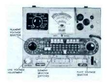
Fig. 4. Commercial Example of an Emission Type Tube Tester.
