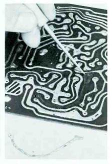
Fig. 3. Conductor Unbonded From Base.
