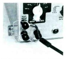
Fig. 6. RF Filter Capacitor Connected Across the Vertical-Input Terminals of an Oscilloscope.
