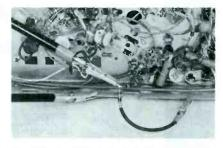
Fig. 5. Pair of Matched Resistors Used in an FM Detector Alignment.
