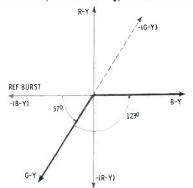
Fig. 7. Phase Relationships Between B-Y, G-Y, and Burst Axes.
