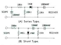
Fig. 10. Two Types of Detector Probes.
