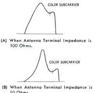
Fig. 8. Attenuation Due to Poor Antenna Design, Tuner With High VSWR, and Transmission Line of Critical Length.
