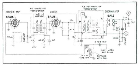
Fig. 3. Schematic of New 4.5-mc Circuit.
