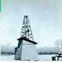
Sample Antenna Under Test. (Rotatable and Tiltable Platform.)
