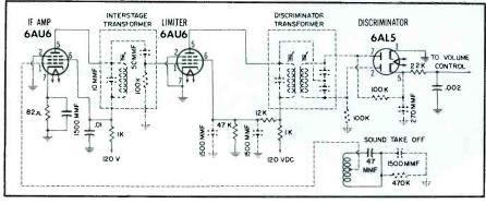
Fig. 1. Schematic of Original RCA Circuit.
