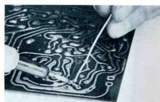
(B) Bonding Wire Bridge to Conductor.
