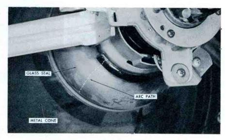
Fig. 2. Arc Path Between Yoke Bracket and Metal Cone of Picture Tube.
