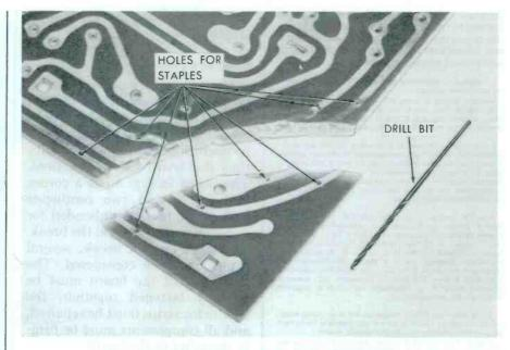
Fig. 6. Holes Drilled to Allow Fastening With Staples.
