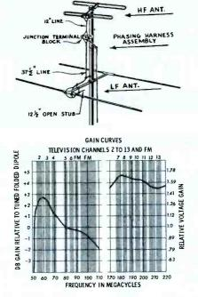
Fig. 3. Mallet Antenna With Separate High Frequency Folded Dipole.
