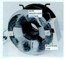
(A) Horizontal Yoke Balancing Coil.
