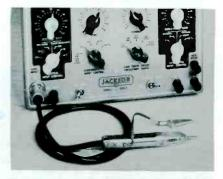
Fig. 9. Detector Probe for Jackson Model CRO-2 Oscilloscope.
