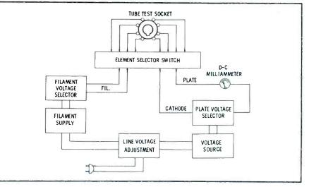
Fig. 3. Simplified Block Diagram of an Emission Type Tester.
