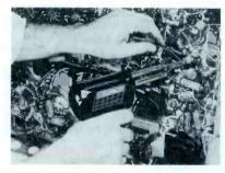
**4 REPAIRING REMOTE-CONTROL TUNING UNITS.** Your Weller Soldering Gun fits neatly into the small spaces between the terminal tabs on telephone-type relay stacks. Also, heat shutoff feature of gun prevents damage to insulation.
