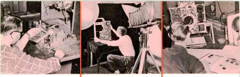
The first step in the processing operation is to remove the chassis from its cabinet. Notes are made on any unusual problems encountered; these are covered in the finished PHOTOFACT Folder.
