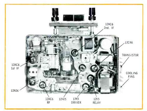
Fig. 4. Photograph Showing Placement of Tubes and Output Transistor in the Motorola Auto Radio. (Courtesy of Motorola, Inc.)
