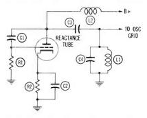
Fig. 3. Basic Circuit of a Reactance Tube.
