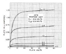
Fig. 2. Plate Current Versus Plate Voltage Curves for a 12F8. Note that the Plate Current Becomes Relatively Independent of the Plate Voltage at About 20 Volts or Less.
