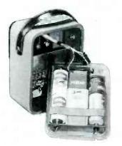
Fig. 5. The Model 78 VTVM with the Back Cover Removed and with the Batteries Exposed.
