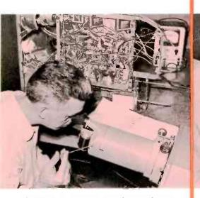
Oscilloscope camera records waveforms at selected reference points in a normally operating television receiver.
