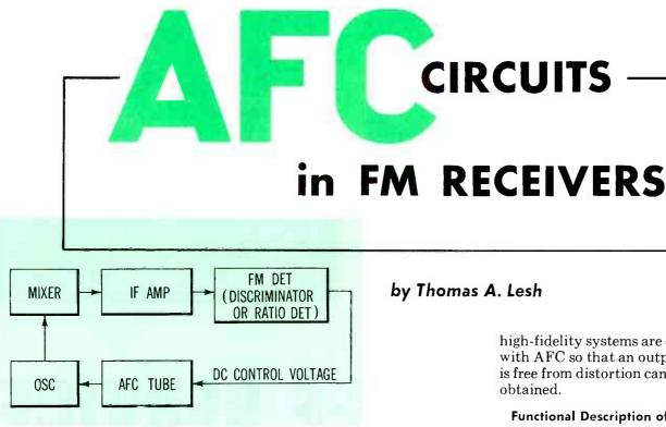
Fig. 1. Block Diagram of the Feedback Path for AFC.
