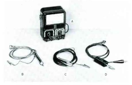
Fig. 1. Some Accessories for an Oscilloscope. (A) Simpson Model 276 Oscilloscope Calibrator. (B) Triplett Low-Capacity Probe. (C) Jackson Low-Capacity Probe. (D) Simpson Peak-to-Peak, High-Frequency Probe.
