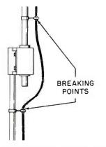
Fig. 2. Possible Breaking Points Near a Rotator.
