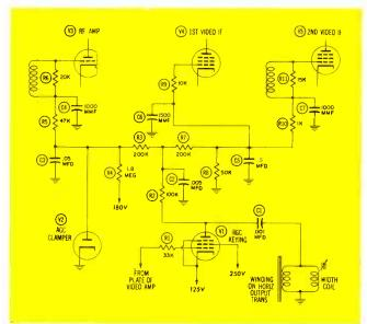
output transformer is separate from all other windings. The cathode of the keying tube is returned to a source of 125 volts. The video signal which is developed in the plate circuit of the video amplifier is used as an AGC input signal. It is passed through the isolating resistor R1 to the grid of V1. The DC voltage on the grid varies according to the strength of the incoming signal, but it is about 100 volts.
