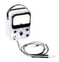
Fig. 4. The Model 78 VTVM by the Precision Apparatus Company, Inc.
