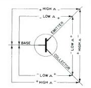
Fig. 5. Ohmmeter Connections for Checking the Power Transistor.
