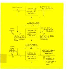
Fig. 1. The Effect of Negative Feedback on a Distorted Signal.
