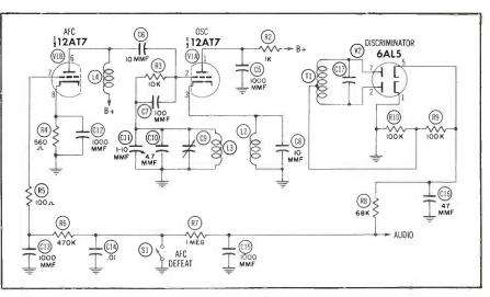
Fig. 5. AFC and Oscillator Circuits of the Harman-Kardon Model D200 Tuner.
