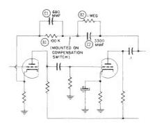
Fig. 3. Circuit of the Damping-Factor Control Used in the Electro-Voice A20C Circlotron Amplifier.
