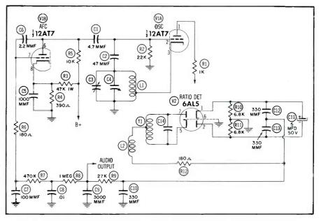
Fig. 4. AFC and Oscillator Circuits of the Packard-Bell Model 10RP1 Tuner.
