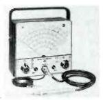
Just announced by Radio Corporation of America is the WV-98A Senior Voltohmyst. This new meter measures DC voltages to 1,500 volts, AC voltages (rms and peak to peak) to 4,200 volts, and resistance to 1,000 megohms.
