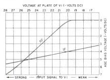
Fig. 3. Graph of the RF and IF Bias Voltages When an AGC Delay Circuit Is Employed.
