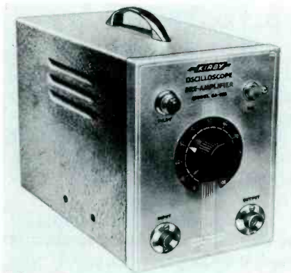
Fig. 3. A Calibrated Oscilloscope Pre-amplifier. (Photograph Courtesy of Kirby Products Corporation.)
