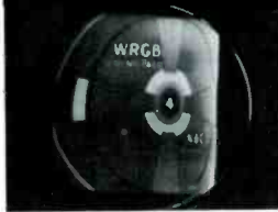
FAULT - Picture compression and stretching. CAUSE - Capacitance value of boost capacitor (connected to linearity coil) too low.
