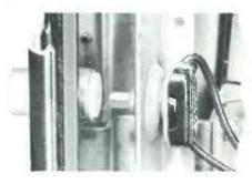
Fig. 9. Push-Button Power Switch Employed in the Motorola Model 21K41R Television Receiver.
