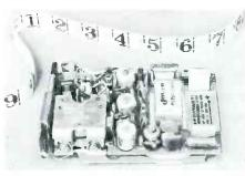
Fig. 8. The Mitchell Model 1103 Transistorized Portable Radio Chassis.
