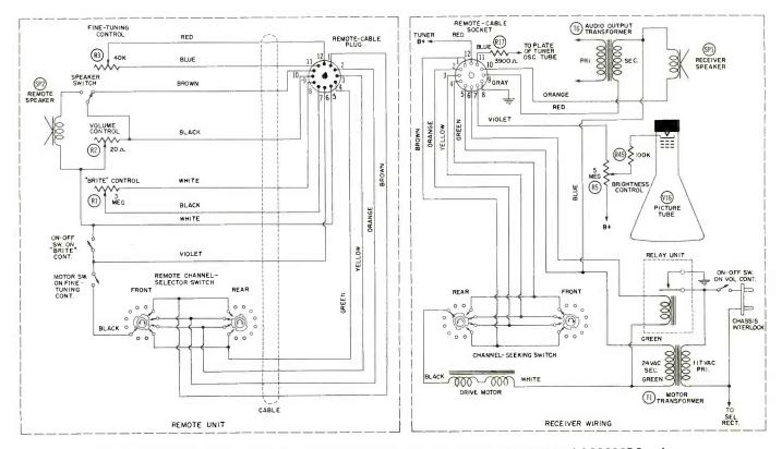
Fig. 3. Schematic Diagram of the Remote-Control System Employed in the Sentinel Model 21121T Receiver.
