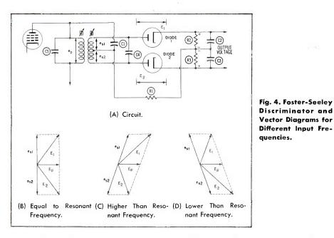
tapped in order that two induced voltages  $e_{S1}$  and  $e_{S2}$ , each with a phase difference of 90 degrees with respect to the primary voltage, may be obtained. The center tap is also connected to the primary circuit through the DC blocking capacitor C1. This connection supplies a reference voltage that is a sample of the primary voltage. The capacitively coupled voltage is not shifted in phase because the reactance of the capacitor is extremely low at the frequency of the primary voltage.
