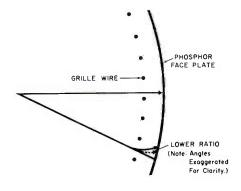
Fig. 3. Drawing Showing the Effect of a Change in the Ratio of the Screen Voltage to the Grille Voltage.
