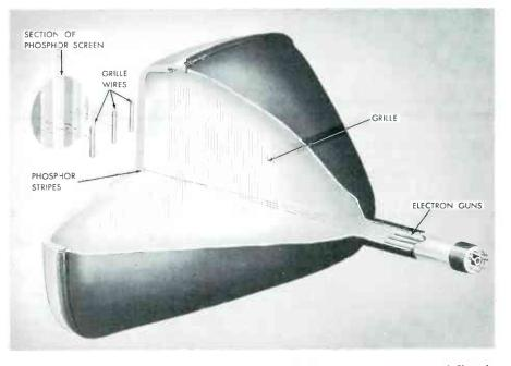
Fig. 1. The Post-Acceleration Color Picture Tube in Development at General Electric Company.
