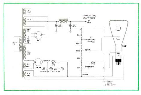
Fig. 2. Partial Schematic Diagram of the Power Supply of the Triplett Model 3441 Oscilloscope.
