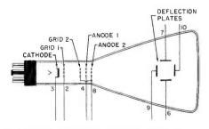
Fig. 1. Control Elements in a 5UP1 Cathode-Ray Tube.
