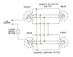
Fig. 4. Simplified Schematic Diagram of the Connections Between the Switches in the Sentinel Remote-Control System.
