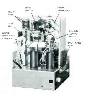
with a connecting plug. The socket for this plug is conveniently located at the rear of the receiver, and it is identified in Fig. 2. The cable from the remote unit must be connected to the receiver in order for the receiver to be operated by the remote controls or by the controls on the receiver itself.
