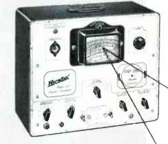
This unit features another HICKOK FIRST—A Non-Parallax shadow type dial provides a 300% magnification of scale, permitting exact settings for most accurate readings, and can be viewed from any angle without error. This entirely new and advanced equipment represents the latest HICKOK achievement in offering complete, fast and accurate solution to TV alignment.
