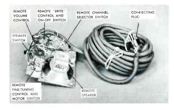
Fig. 1. Remote-Control Chassis and Connecting Cable Employed in the Sentinel Model 21121T.
