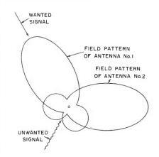
Fig. 4. Field Patterns of Antennas Arranged So That Interference From the Back Will Be Rejected.
