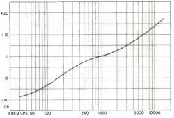
Fig. 2. RIAA Recording Curve.
