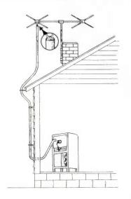
Fig. 1. Improper Installation of Lead-in Wire.
