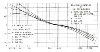
Fig. 4. Comparison of Standard RIAA Playback Curve With Some Curves Used Before Standard Curve Was Adopted.
