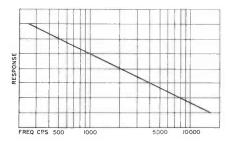
Fig. 1. Typical Response Curve Showing Change in Amplitude With Change in Frequency When Velocity Remains Constant.
