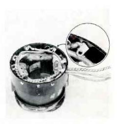
Fig. 2. Short Between Wire and Terminal in Deflection Yoke.
