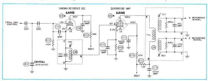
Fig. 12-12. Circuit of the 3.58-Mc Oscillator and Quadrature Amplifier in the RCA Victor Model CT-100 Color Receiver.
