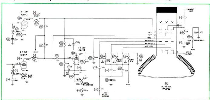
Fig. 12-2. Matrix Section and Circuits Associated With the Picture Tube in the Motorola Model 19CT1 Color Receiver.
