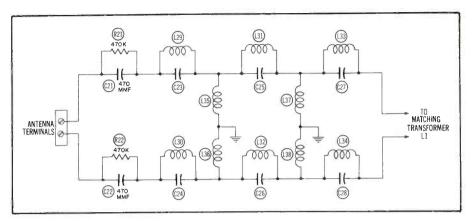
Fig. 4. Schematic Diagram of Tuner Input Circuit.
