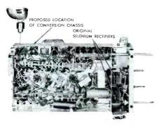
Fig. 11. Location of Original Rectifiers in General Electric TV Receiver and Holes Being Drilled at Proposed Location on Conversion Chassis.
