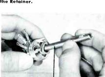
Fig. 6E. The Outer Shaft Is Placed Over the Inner Shaft.
