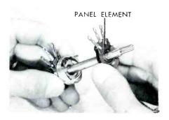
Fig. 6F. The Panel Element Is Slipped Over the Outer Shaft.
