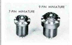
Fig. 12. Test Adapters for Tube Sockets.
