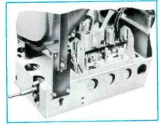
Fig. 19. TV Tuner Which Employs a High-Low Band Switch.
