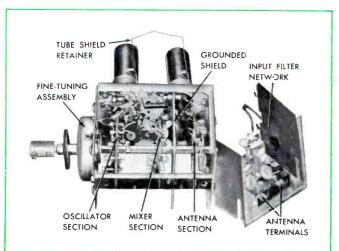
Fig. 2. VHF Tuner With Cover Removed.
