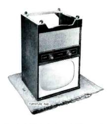
Fig. 6. Position of Cabinet While Casters Are Being Mounted.
