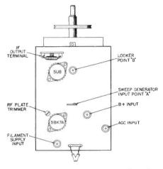
Fig. 3. Top View of Tuning Unit Showing Various Test Points.
