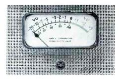
Fig. 3. VU Meter Used on Ampex Model 600 Magnetic Tape Recorder. Meter Is Mounted in Perforated Metal Front Panel of Recorder.
