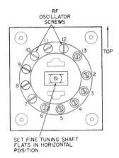
Fig. 6. Front View of Tuning Unit Illustrating RF Oscillator Adjustments.
