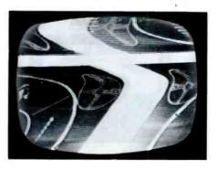
Fig. 21. Negative Picture and Loss of Synchronization.
