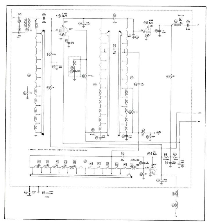
Fig. 3. Schematic Diagram of a Switch Type of Tuner With a Pentode RF Stage.
