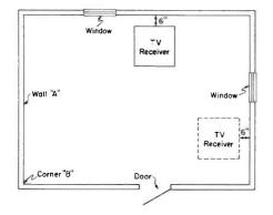
Fig. 1. Receiver Positions for Proper Ventilation.
