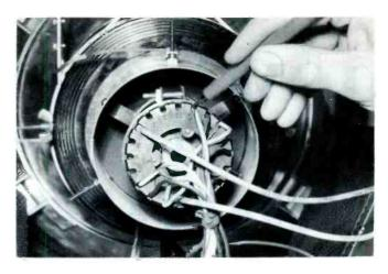
Fig. 12-3. A Needle-Point Probe Inserted at the Picture-Tube Socket to Measure Voltage.
