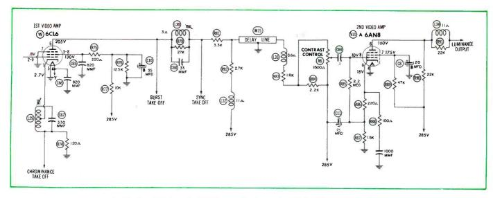
Fig. 12-1. Luminance Channel in the RCA Victor Model CT-100 Color Receiver.
