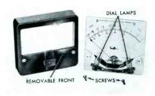
Fig. 4. Simpson 4-Inch Model 142 VU Meter With Front Removed to Show Access to Dial Lamps.
