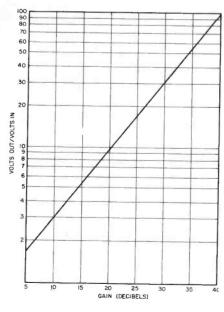
Fig. 2. Conversion Chart for Finding the Gain of a Transistor in an Amplifier After Measuring Input and Output Voltages.
