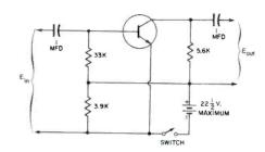
Fig. 1. Circuit for Testing Transistors Used in Amplifier Stages. Connections Are Shown for an *n-p-n* Type of Transistor.
