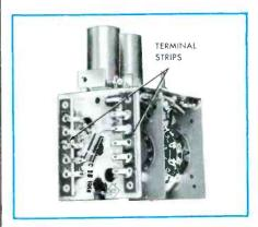
(B) Terminal Strips on Rear of Tuner.
