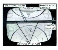
Fig. 23. Normal Vertical-Blanking Bar Obtained by Adjusting Vertical-Hold Control.
