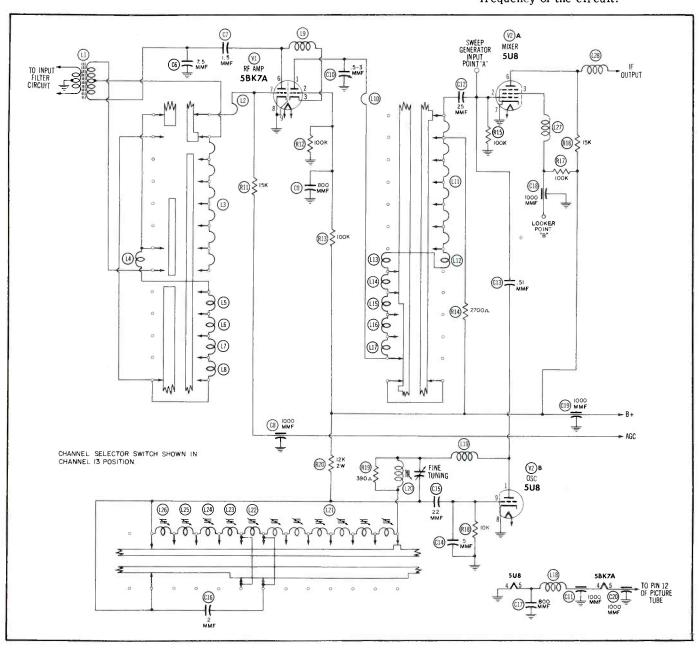
Fig. 5. Schematic Diagram of Zenith 12-Position VHF Tuner.
