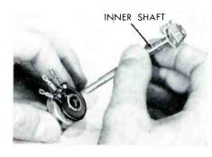
Fig. 6B. The Inner Shaft Is Inserted in the Rear Element.
