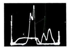
Fig. 3. Response Curve Showing Interference Pickup Caused by the Use of Long Unshielded Leads to the Chromatic Amplifier.
