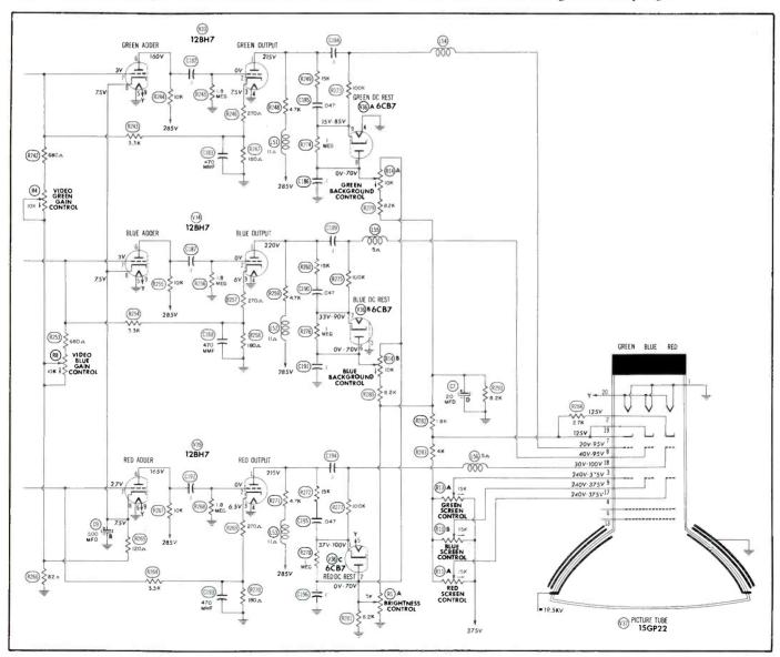
Fig. 12-4. Matrix Section and Circuits Associated With the Picture Tube in the RCA Victor Model CT-100 Color Receiver.
