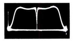
Fig. 2. Response Curve Representing the Output Obtained From Simpson Chromatic Amplifier and Probe When These Are Used With a Simpson Model 480 Genescope.
