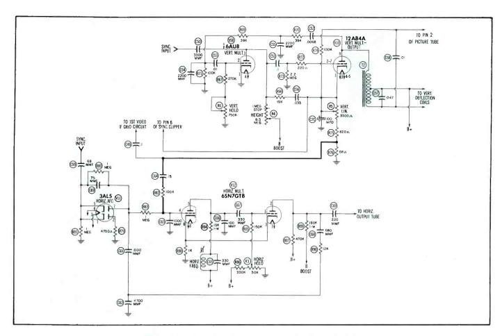
Fig. 7. Bend-Correcting Circuit Used in Zenith Chassis 16T20.
