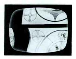
Fig. 17. Loss of Synchronization.
