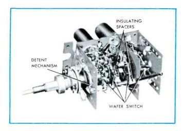
Fig. 5. Interior of Switch Type of Tuner.
