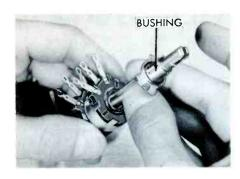
Fig. 6G. The Bushing Is Slipped Into Place Over the Outer Shaft.
