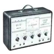
Fig. 5. Triplett Model 3439 Color-Bar Gen-
