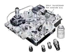
Fig. 2. High-Voltage Area Ready to Be Sprayed With Acrylic Plastic.
