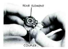
Fig. 6A. The Rear Element Is Placed on Coupler.
