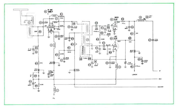
Fig. 2. Schematic Diagram of a Turret Type of Tuner With a Cascode RF Stage.
