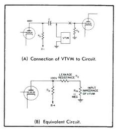
Fig. 13. Setup for Testing a Coupling Capacitor for Leakage Resistance.
