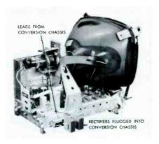
Fig. 12. Completed Installation for Plug-in Rectifiers.
