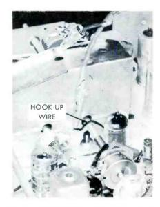
(C) At Loose End of Hook-up Wire With Other End Looped Around the Pin of the Control Grid.
