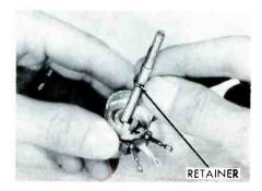
Fig. 6C. The Retainer is Placed on the Inner Shaft.
