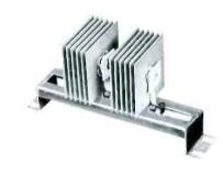
Fig. 9. View of Conversion Chassis With Rectifiers in Place.
