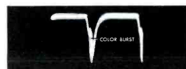
Fig. 27. Signal at Plate of Burst Amplifier.
