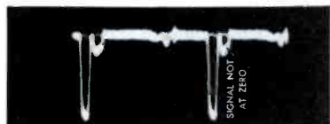
Fig. 17. Signal at Plate of I-Demodulator Illustrating Improper Cancellation of Q Signal.
