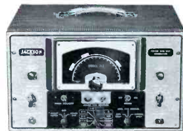
Fig. 7. The Jackson Model 712 Color Bar/Dot Generator.
