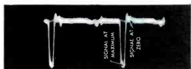
Fig. 16. Signal at Plate of I-Demodulator Illustrating Proper Cancellation of Q Signal.
