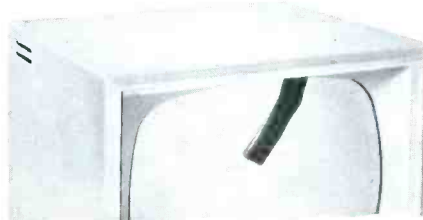
Fig. 12. Dust Seal Out of Place.
