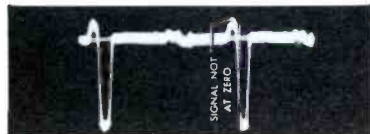
Fig. 19. Signal at Plate of Q-Demodulator Illustrating Improper Cancellation of I Signal.
