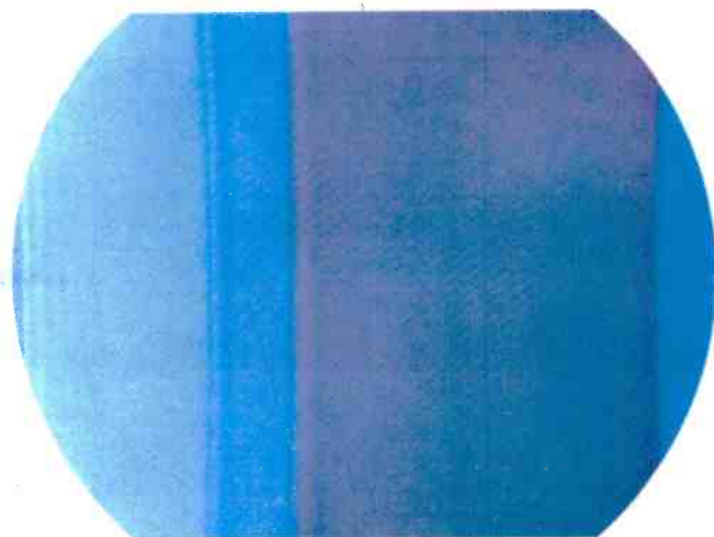
Fig. C-9. Q and I Pattern Resulting From Misadjustment of Quadrature Transformer. Phase Difference of CW Reference Signals Is More Than 90 Degrees.
