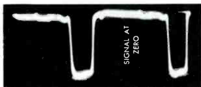
(A) With Proper Cancellation During Transmission of an I Bar.
