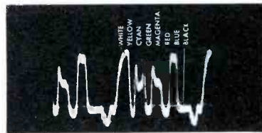
Fig. 25. Signal at Grid of Blue Gun.
