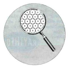
Fig. 9-3. Arrangement of Phosphor Dots on the Screen of the Color Picture Tube (As Seen Under Magnifying Glass).
