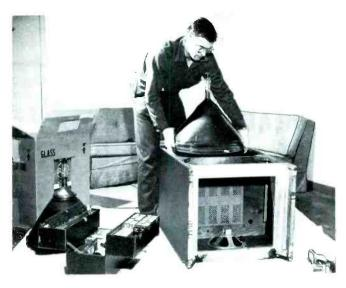
Fig. 7. Replacing a Picture Tube in the Custamer's Home.
