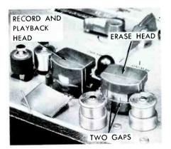
Fig. 2. High-Frequency Erase Head Used in Magnecord Model M30 Tape Recorder.
