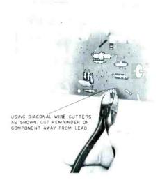
Fig. 6. Removing Resistor From Leads. (Courtesy of Admiral Corp.)
