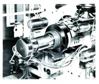
Fig. 6. Modified Centering Assembly in Place on the Neck of the Tube.
