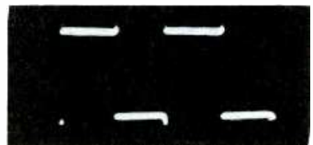
Fig. 2. Output Signal From the Electronic Switch With Both Amplifiers Set for Zero Gain.
