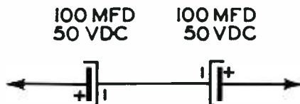
Fig. 4. Hookup for Double-Capacitor Substitution Unit.
