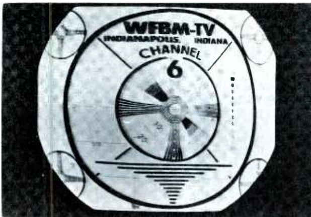
Fig. 9B. The Effect of the Deflection Wave in Fig. 9A on a Picture.
