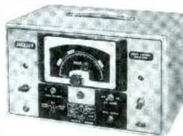
Fig. 8. Jackson Model 712 Color Bar/Dot Generator.
