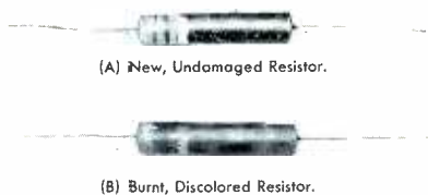
Fig. 5. Effects of Excessive Power Dissipation.
