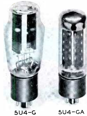
Fig. 3. Full-Wave Power Rectifier 5U4G and the New 5U4GA. (Samples Courtesy of General Electric Co.)
