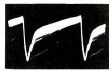
(A) Horizontal Oscillator Operating at Sync-Pulse Frequency.
