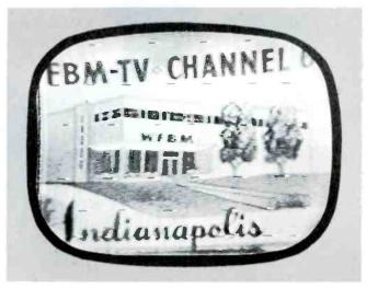
Fig. 6. Ignition Interference.
