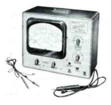
Four panel controls are provided as follows: FUNCTION SE-LECTOR, RANGE SELECTOR, ZERO ADJ, and OHMS ADJ. The function selector positions are: OFF, +DC, -DC, AC, and OHMS.
