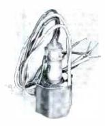
Fig. 4. A Horizontal Dynamic-Convergence and Dynamic Focus Transformer.
