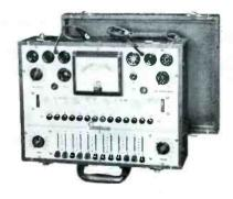
The BIAS control is a vernier adjustment for the tube-operating voltages selected by the toggle switches. One toggle switch selects any of six meter sensitivity ranges, and the RANGE control provides a vernier adjustment of the range selected.
