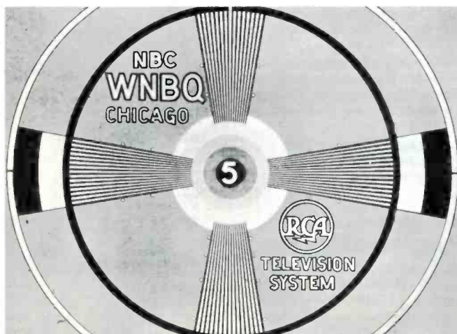
Fig. 5. A Typical Test Pattern. Courtesy of NBC
