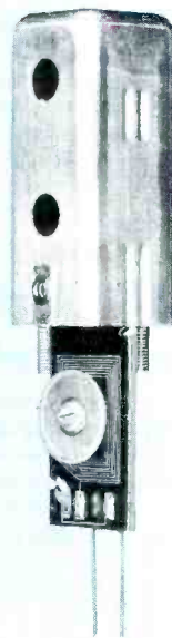
Fig. 3. A Printed-Circuit Coil Partially Removed From Its Shield Can.
