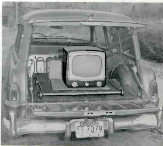
Fig. 5. Dolly in Position for Travelling.
