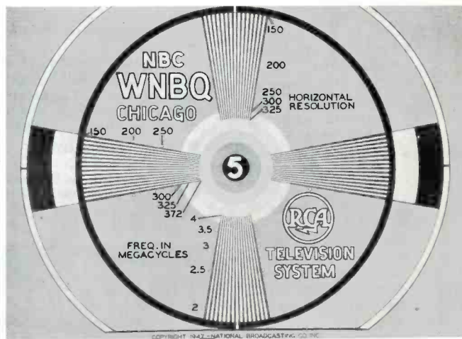
Fig. 6. Same Test Pattern as Fig. 5, With Resolution Shown at Various Points Along Wedges. Courtesy of NBC
