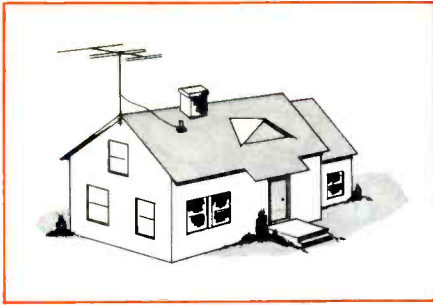
Fig. 10. Antenna Should Not Be Grounded to Sanitary Vent Pipe. (Courtesy NFPA.)
