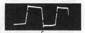
Figure 10. Effects of Various Values of Buffer Capacitors; Too small (A), Too large (B), and Correct Value (C).
