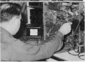
2. LOCATING THE SHORT -- With Loadchek you can quickly check the shorted side, part by part, without laying down tools or picking up test leads. Here, the trouble was a short in the transformer, spotted without having to warm up set. Overloads are round the same way.
