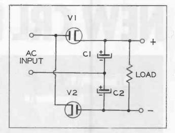
Figure 5. A Full-Wave Voltage-Doubler Circuit.
