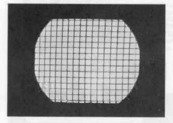
Figure 3. Crosshatch Pattern Produced by Videometer.
