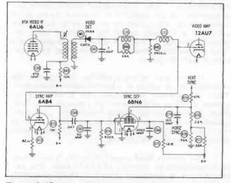
Figure 6-18. Sync Circuit Employing Type 6BN6 for Sync Separation.
