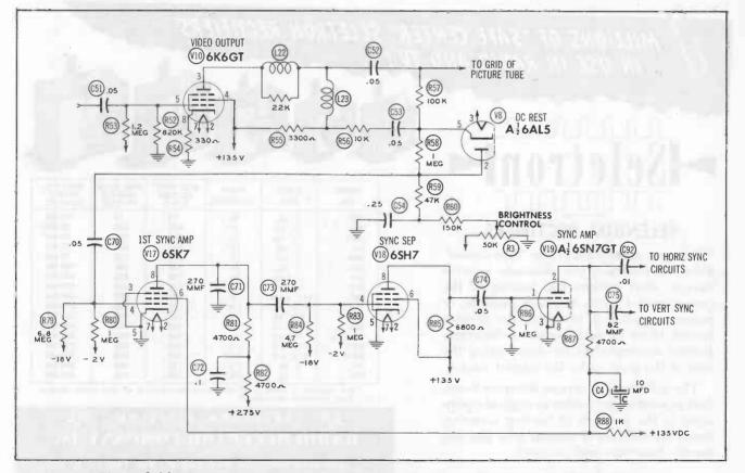
Figure 6-24. Combination DC Restorer and Sync Separator Circuit Used Commercially.
