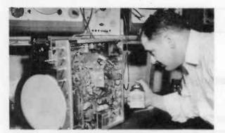
Because of its high dielectric strength, Krylon helps prevent corona. Here technician Bernard Vanella "Krylon-izes" high voltage coil and insulation, the socket of the high voltage rectifier, component parts of the rectifier circuit.
