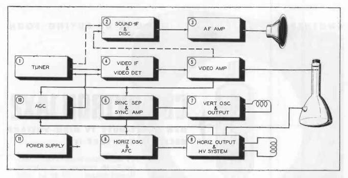
Figure 6. Block Diagram of Typical Receiver,
