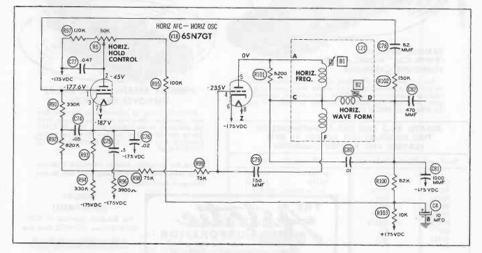
Figure 2. An AFC Circuit Similar to that of Figure 1, but with Apparently Differing Voltage Values.
