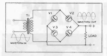
Figure 3. A Bridge Type Rectifier Circuit.
