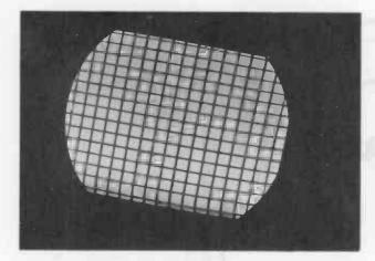
Figure 4. Pattern Resulting from Improperly Positioned Yoke.
