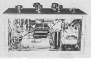
Figure 4. Bottom View of Preamplifier and Control Unit.
