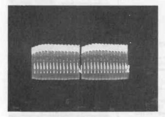
Figure 7. Overloading in RF or IF Stages Causing Sync Compression.
