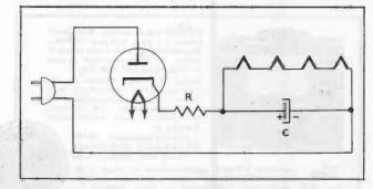
Figure 2. Filament circuit of an AC-DC Battery Portable.
