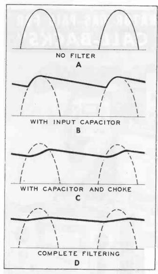
Figure 6. Waveforms with Various Types of Filter Networks.
