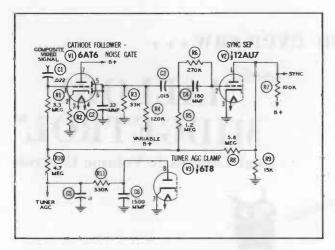
Figure 3. Noise Gate and Tuner AGC Circuits.
