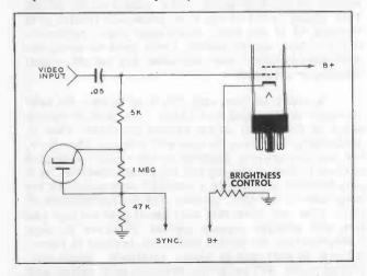
Figure 6-20. Combination DC Restorer and Sync Separator Using Diode.
