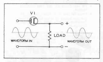
Figure 1. A Typical Half-Wave Rectifier Circuit.
