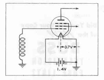
Figure 3. "A" Battery Connections to a 1.5 Volt Tube.
