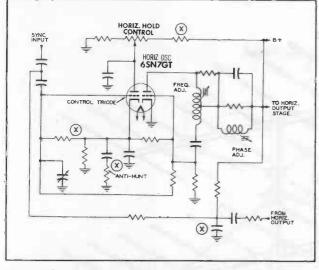
Figure 2. Typical Synchroguide Horizontal Lock System.
