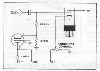
Figure 6-21. Combination DC Restorer and Sync Separator Using Triode.
