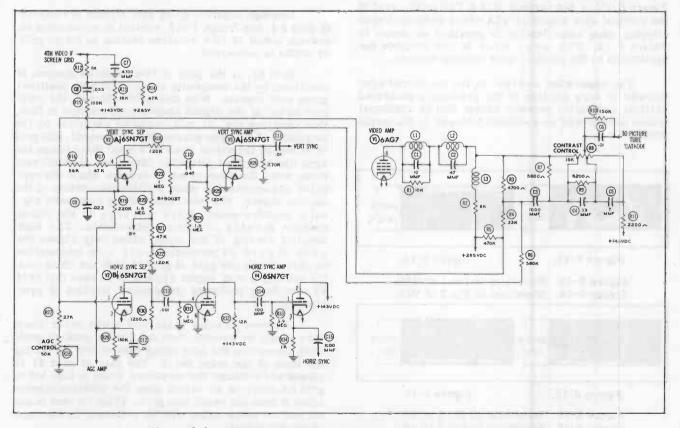
Figure 6-8. Separate Vertical and Horizontal Sync Separator Stages.
