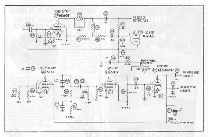
Figure 9. Typical 3-Stage Sync Separator Circuit.
