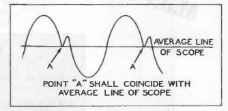
Figure 4. Waveform Present at the Horizontal Oscillator Cathode.
