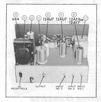
Figure 3. Top View of Preamplifier and Control Unit.
