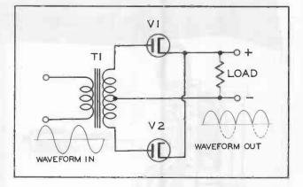
Figure 2. A Full-Wave Rectifier Circuit.
