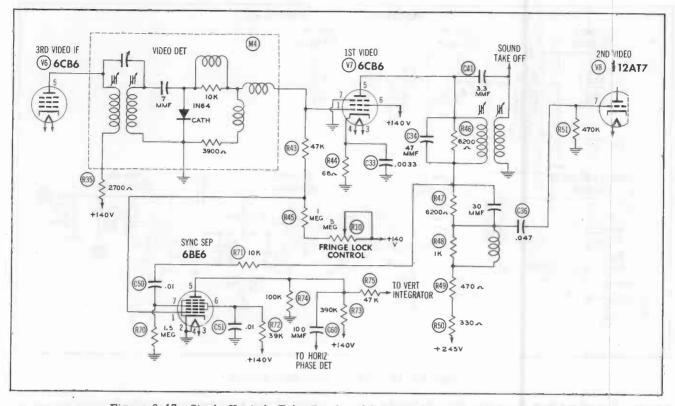
Figure 6-17. Single Heptode Tube Employed for Sync Separation and Limiting.
