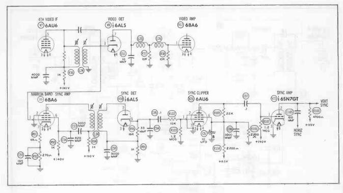
Figure 6-19. Narrow Band Sync System.
