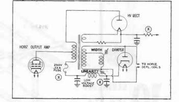
Figure 3. Horizontal Output and High Voltage Supply.
