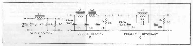
Figure 7. Typical Filter Network Circuits.
