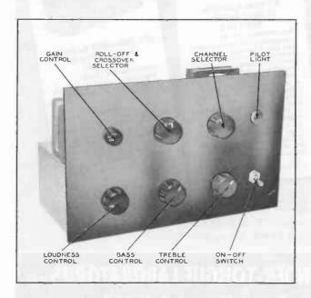
Figure 1. Panel View of Preamplifier and Control Unit.
