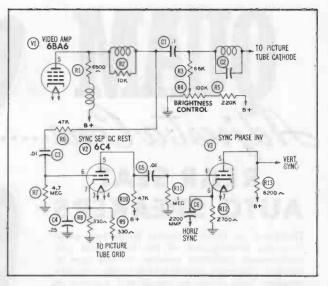
Figure 6-23. A commercial Type DC Restorer and Sync Separatór Circuit.
