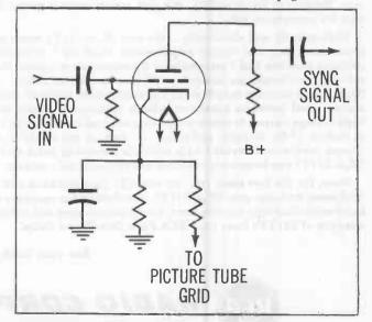
Figure 6-22. Combination DC Restorer and Sync Separator (Cathode Bias Method).
