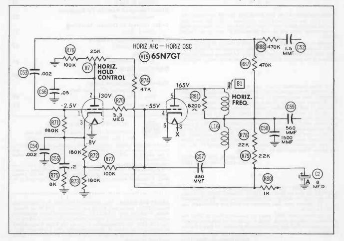
Figure 1. A Representative Pulse-Width AFC Circuit.
