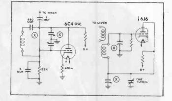
Figure 1. Typical Local Oscillator Circuits.
