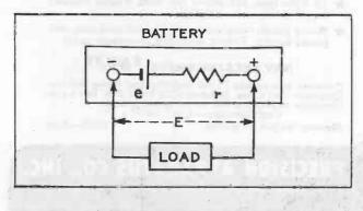
Figure 1. Equivalent Circuit of a Battery.
