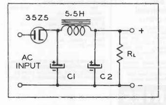
Figure 8. Circuit of Power Supply Used to Obtain Data Included in this Article.
