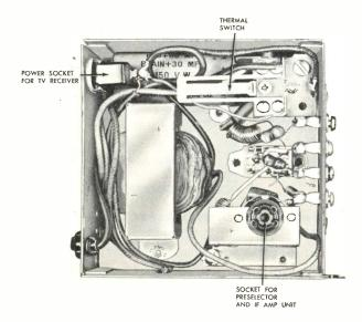
Figure 2. Rear View of Power Supply Section of Ampli-Verter.
