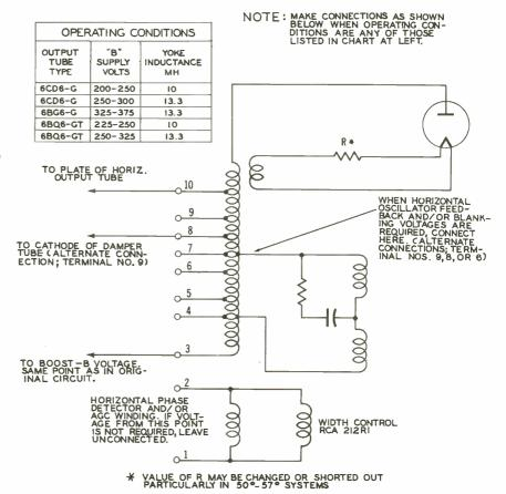
Figure 9. One of Several Schematic Guides Packed with the RCA 232T1 Horizontal Output Transformer.
