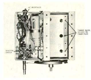
Figure 10. Top Chassis View of Granco Converter.
