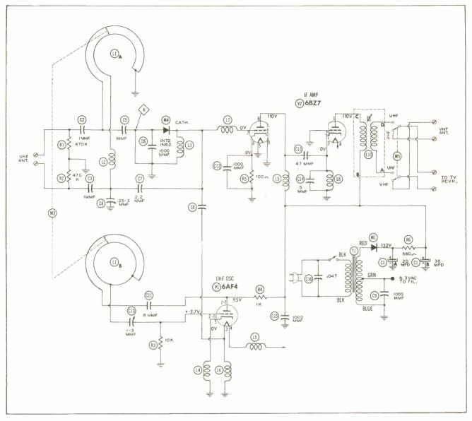
Figure 8. Schematic of Bogen UHF Converter (Model UCT).
