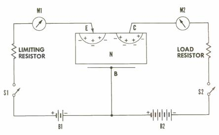
Figure 6. Basic Point-Contact Transistor Circuit.
