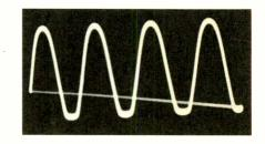
Figure 3. Sample Waveform Indicating the Presence of a Signal.
