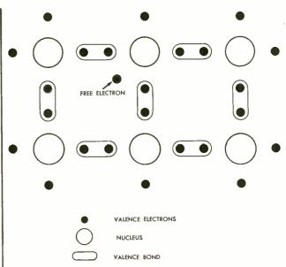
Figure 2. Substitution With One Atom Having Five Valence Electrons.
