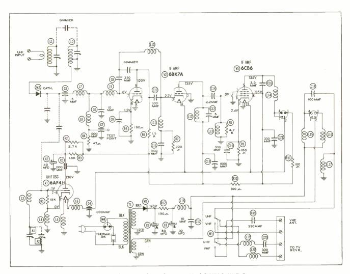
Figure 4. Schematic of Ampli-Verter Model BTU-1 UHF Converter.
