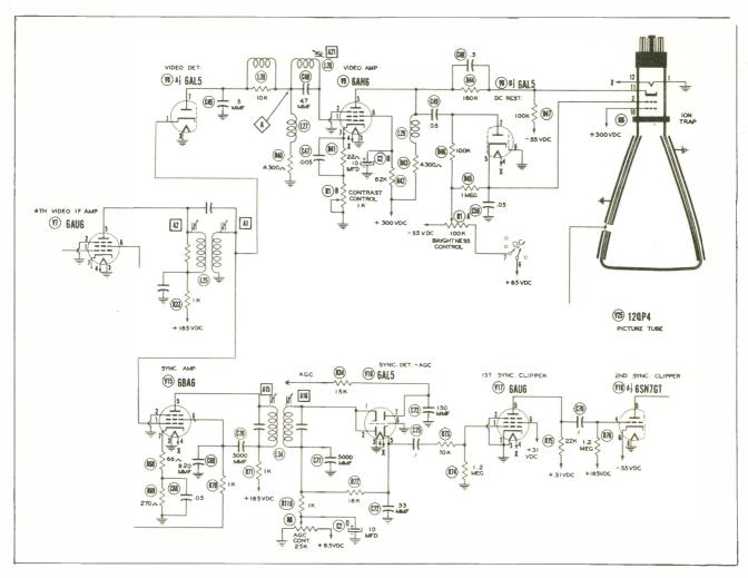
Figure 1. Sync Separator System in the DuMont RA-111A TV Receiver.
