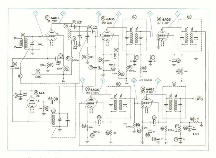
Figure 2. Partial Circuit of a Typical FM Receiver, Showing Test Points 6 to 15 Discussed in Text.
