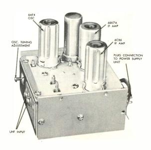
Figure 3. Preselector and IF Section of Ampli-Verter.
