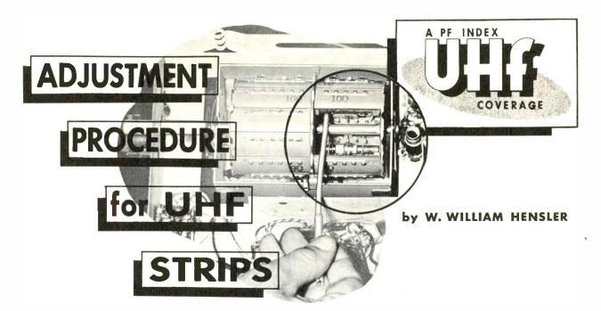
A very popular method of converting the VHF receiver to UHF operation is provided through the use of Standard Coil UHF Strips in receivers having tuners of that manufacture. The conversion procedure consists of removing a pair of VHF strips of an unused channel, and replacing them with UHF strips designed to provide reception on the desired UHF channel.
