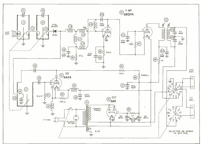
Figure 12. Schematic of Granco Converter.
