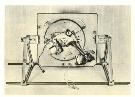
Figure 1. Mounting Rack for Holding Record Changer.
