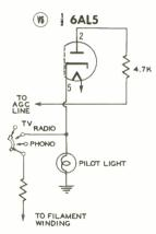
Figure 1. Partial Schematic from CBS-Columbia Showing System Used for Disabling Video IF When Using AM
