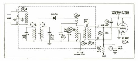
Figure 1. Input Circuit of the Standard Coil UHF Strip.
