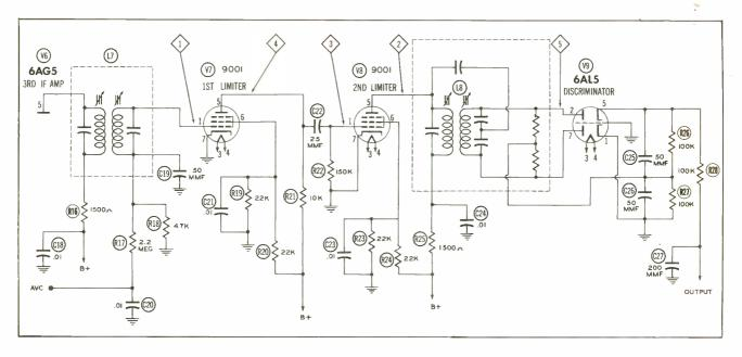
Figure 1. Partial Circuit of a Typical FM Receiver, Showing Test Points 1 to 5 Discussed in Text.
