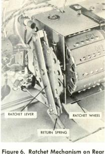
Figure 6. Ratchet Mechanism on Rear of Tuner in Kaye Halbert 263.
