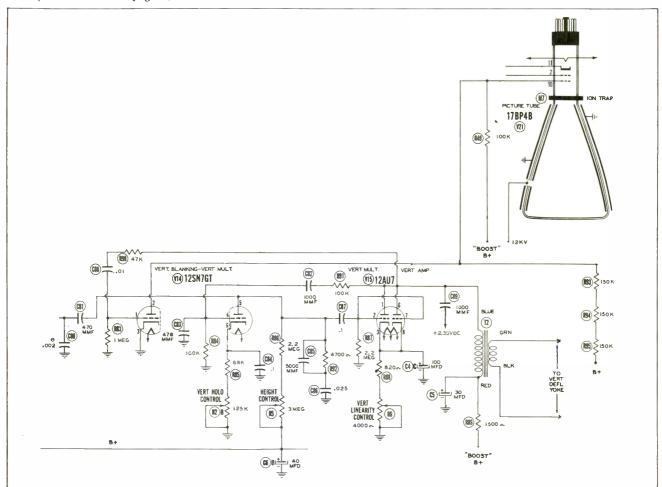
Figure 2. Vertical Blanking Circuit Employed in the GE Model 17C103 TV Receiver.
