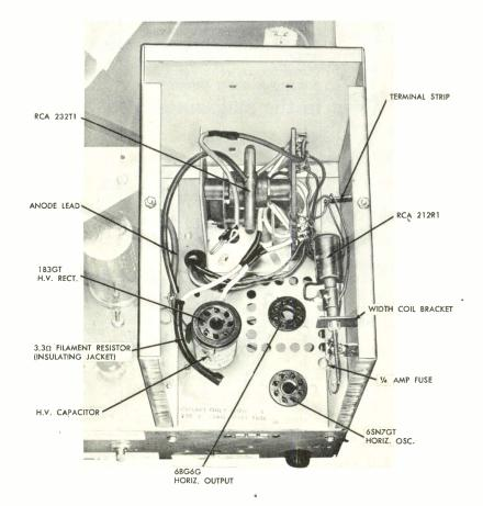
Figure 11. High Voltage Compartment After Transformer Replacement.
