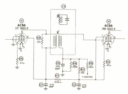
Figure 7. Partial Schematic of Magnavox MV310M-1 Showing 1st and 2nd Video IF Stages Connected in Series.
