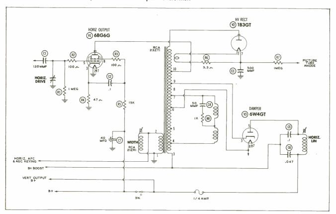
Figure 10. Schematic of Horizontal Deflection Output Section After Transformer Replacement.
