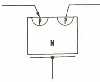
Figure 5. Point-Contact Transistor Construction.
