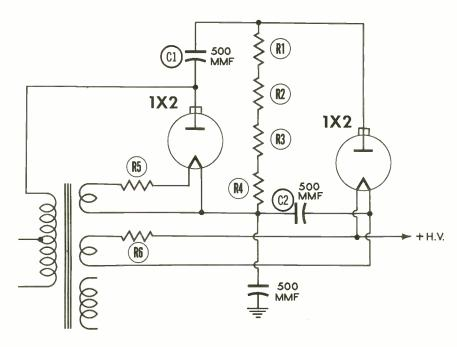
Figure 3. A Typical Voltage Multiplier Circuit.
