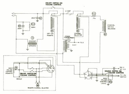
Figure 3. Schematic of Remote Control Head and Relay Circuit Used with Kaye Halbert 263.
