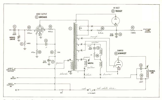
Figure 7. Schematic of Horizontal Deflection Output Section Before Transformer Replacement. (Script Notes Were Made by the Technician.)
