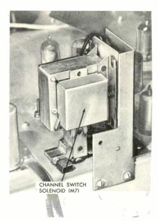
Figure 5. Channel Selector Solenoid for Changing Stations in Kaye Halbert 263.
