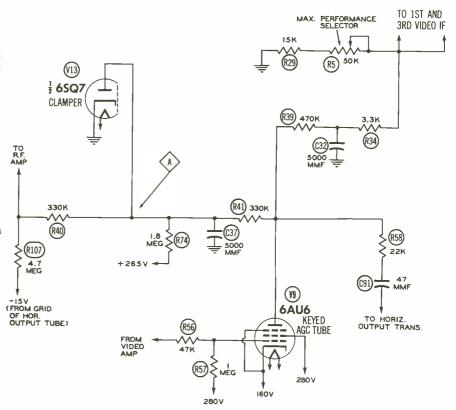
Figure 4. The AGC System in the Hoffman Model 21B116 TV Receiver.
