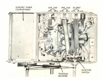
Figure 7. Bottom Chassis View of Bogen UHF Converter (Model UCT).
