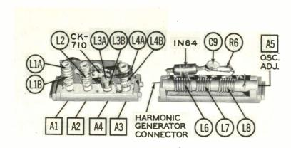
Figure 2. A Set of Standard Coil UHF Strips Showing Location of Components and Adjustment Points.
