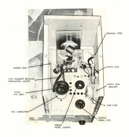
Figure 8. High Voltage Compartment Before Transformer Replacement.
