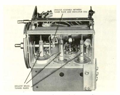
Figure 13. Tuning Slugs Attached to Tuner Plate.
