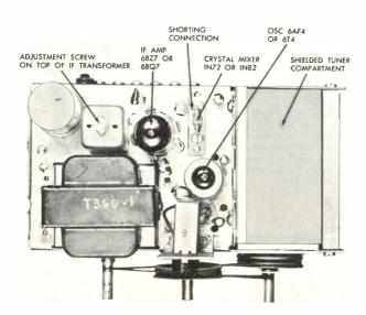
Figure 6. Top Chassis View of Bogen UHF Converter (Model UCT).
