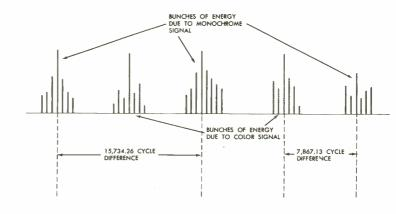
Figure 1. Concentration of Energies of the Interleaved Chrominance and Luminance Signals.
