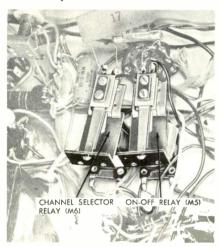
Figure 4. View of Power and Channel Selector Relays Mounted on Under Side of Chassis of Kaye Halbert 263.
