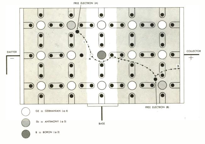
Figure 7. Enlarged Portion of Junction Transistor Showing Carrier Action.
