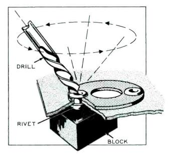
Figure 3. Removing a Rivet by Drilling.
