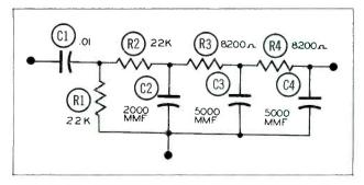
Figure 13. Schematic of Unit Shown in Figure 12.
