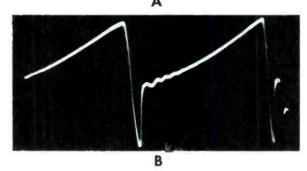
Figure 2. Waveforms Typical of Those Found on the Control Grids of Horizontal Sweep Amplifiers.
