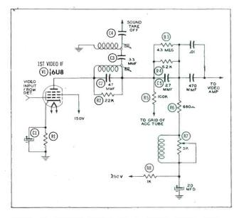
Figure 8. Partial Schematic of Zenith Video Amplifier Stage Containing Variable Frequency Response Provision,
