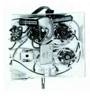
Figure 7. Coupling Circuit Wired Into Small Radio.
