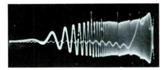
Figure 7. Output of Variable Reluctance Cartridge.
