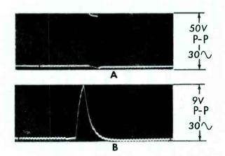
Figure 9. (A) Input to Integrator Network. (B) Output of Integrator Network.
