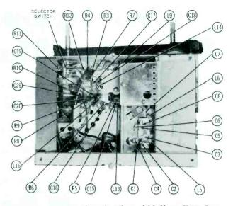
Figure 8. Bottom Chassis View of Mallory UHF Converter. Early Version. (Before Serial #200,000).
