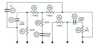
Figure 14. Schematic of Special Audio Compensating Printed Circuit.
