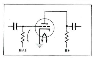
Figure 1. Direction of Grid Current Flow in a Normal Operating Tube When the Grid is Driven Positive by Signal Components.
