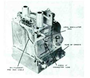
Figure 5. The Zenith Turret Tuner Employed on Chassis 21K20.
