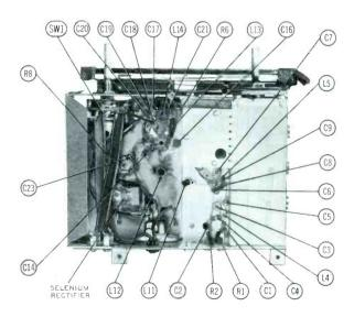
Figure 12. Bottom Chassis View of Mallory Converter. Late Version.
