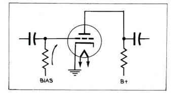
Figure 2. Direction of Grid Current Flow When the Grid Emits Electrons.
