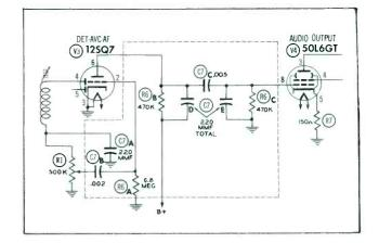
Figure 6. Partial Schematic Showing Incorporation of Printed Coupling Circuit.
