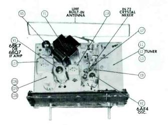
Figure 7. Top Chassis View of Mallory Converter. Early Version. (Before Serial #200,000).
