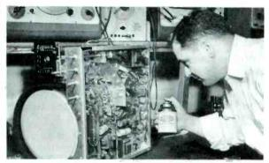
Because of its high dielectric strength, Krylon helps prevent corona. Here technician Bernard Vanella—on the staff of dealer Mort Farr, Philadelphia—"Krylon-izes" high voltage coil and insulation, the socket of the high voltage rectifier, component parts of the rectifier circuit.
