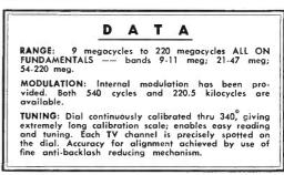
The only single easily portable instrument that provides for testing and alignment of: Front Ends, IF's, Horizental and vertical linearity, syncs, sweeps, size, position, focus coil, deflection coil, ion trap.
