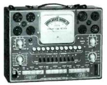
In the Model 115 "Challenger" Tube Tester, the famous Jackson Dynamic® test principle is employed. Separate voltages are applied to each tube element. Tests can be made under actual use conditions.
