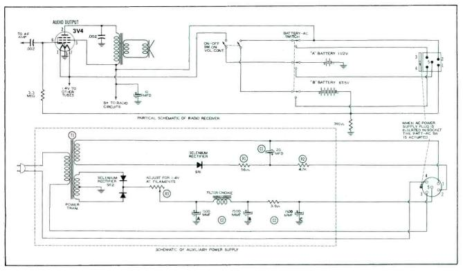
Figure 4. Schematic of Westinghouse Model H-377 Auxiliary Power Supply.
