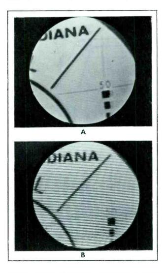
Figure 1. Expanded Partial Photograph of a Test Pattern Illustrating (A) Good Interlace and (B) Poor Interlace.
