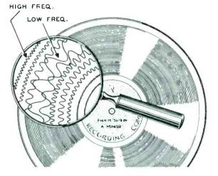
Figure 1. Cver-Modulation of Grooves at Low Frequencies.
