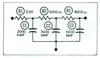
Figure 8. Typical Integrator Network.
