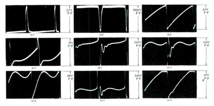
Figure 7. Waveforms Observed in Synchroguide\* Circuit of Figure 6. Peak-To-Peak Voltages are Indicated as They Were Found on the Particular Receiver Upon Which These Tests Were Taken. Considerable Variation Will be Found With Different Receivers. (Oscilloscope Sweep Rate is 7875 cps.)
