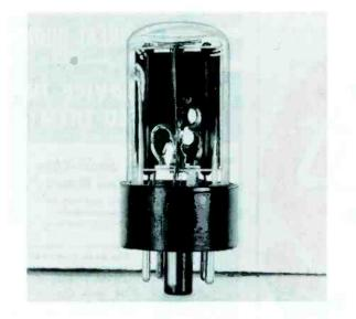
Figure 3. A Photo of a Rectifier Tube Damaged as the Result of Warped Plates.
