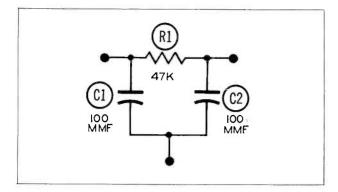
Figure 2. Schematic of Diode Filter Unit Shown in Figure 1.
