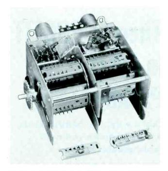
Figure 7. Turret Drum of Zenith Tuner With a Pair of Strips Removed.
