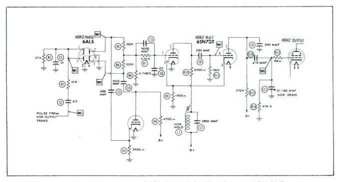
Figure 4. Schematic of Typical Horizontal AFC System Using Phase Detector and Multivibrator.
