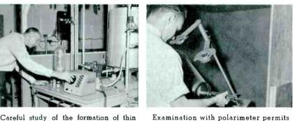
Examination with polarimeter permits careful control of strains for superior glass-to-metal sealing.
