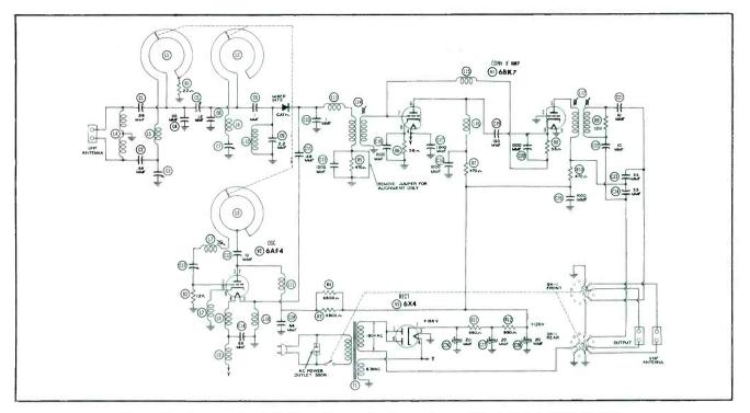
Figure 9. Schematic of Mallory Converter Using Type 6BK7 IF Amplifier Tube.
