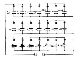
Figure 2. A Suitable Capacitor Substitution Box.
