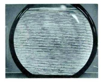
Figure 3. Photograph of CR Tube Image With Horizontal Oscillator Operating at Random Frequencies.
