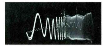
Figure 9. Output of Variable Reluctance Cartridge Through Preamplifier and Control Unit.
