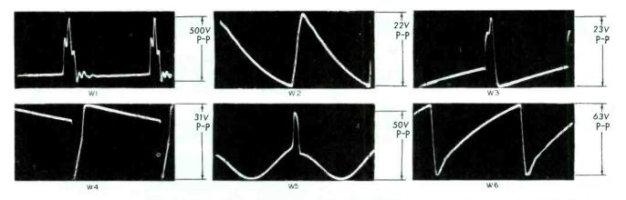
Figure 5. Waveforms Observed in Phase Detector and Multivibrator Circuits of Figure 4. Peak-To-Peak Voltages are Indicated as They Were Found on the Particular Receiver Upon Which These Tests Were Taken. Considerable Variation Will be Found With Different Receivers. (Oscilloscope Sweep Rate is 7875 cps.)
