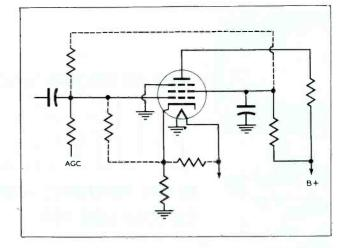
Figure 5. Leakage Paths Which May Exist in a Tube or Tube Socket.
