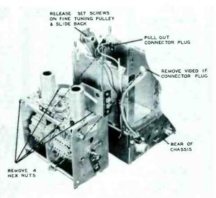
Figure 6. Zenith Tuner Removed From Chassis.
