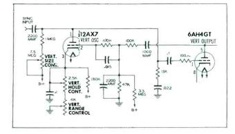
Figure 9. Vertical Range Control Employed in Zenith Chassis.
