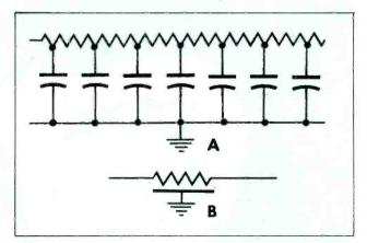
Figure 11. (A) Ladder Type Integrator Employing an Infinite Number of Capacitors and Resistors. (B) Simplified Schematic of the Circuit of (A).
