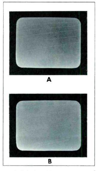
Figure 2. Visible Vertical Retrace Lines Illustrating<sup>\*</sup> (A) Good Interlace and (B) Poor Interlace.
