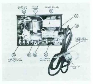
Figure 3. Westinghouse Model H-377 Auxiliary Power Supply (Cover Removed).
