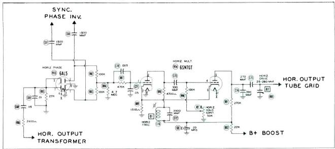
Figure 4. Typical Phase Detector and Multivibrator Horizontal AFC System.
