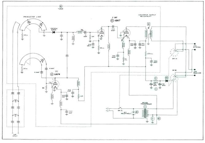
Figure 17. Schematic of Regency Converter.
