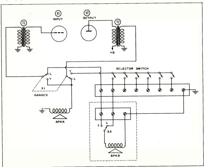
Figure 1. Typical Intercommunication System With Remote Unit.
