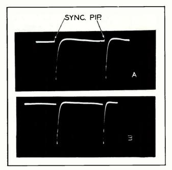
Figure 3. Waveforms at Point W2. (A) Normal. (B) With Open Capacitor C1.
