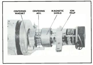
Figure 3. Centering Magnet, Magnetic Shield and Ion Trap Used on Picture Tube.
