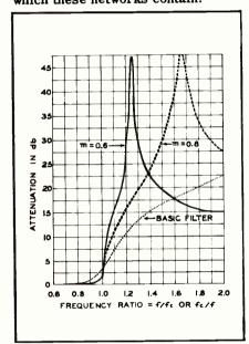
Figure 4. A Comparison of the Effectiveness of Basic and M-Derived Filters.
