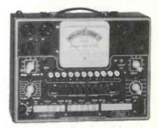
In the Model 115 "Challenger" Tube Tester, the famous Jackson Dynamic® test principle is employed. Separate voltages are applied to each tube element. Tests can be made under actual use conditions.
