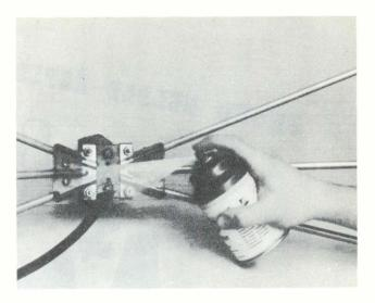
Figure 5. Spraying the Antenna Resistor with Plastic.
