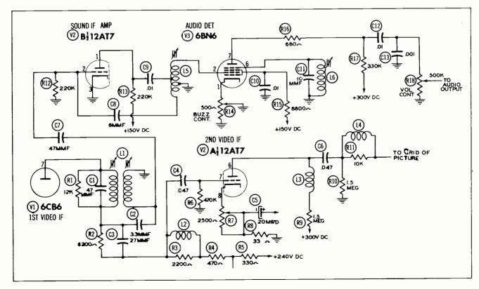
Figure 5. Gated Beam Audio Detector Circuit.
