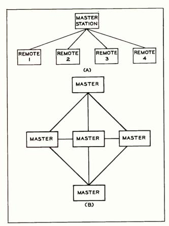
Figure 2. Intercommunication Unit Arrangements. (A) Master and Remotes. (B) All Master Units.
