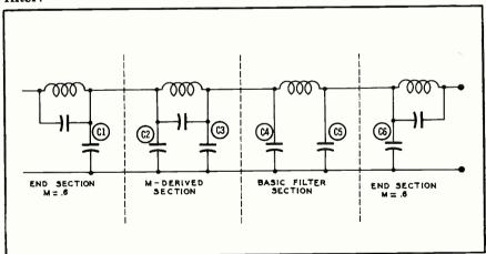
Figure 6. The Complete Filter, Containing Two End Sections, an M-Derived Section, and a Basic Filter.
