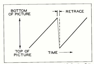
Figure 7. Current Wave in Vertical Deflecting Coils Showing its Relation to Movement of Electron Beam on Picture Tube Screen.
