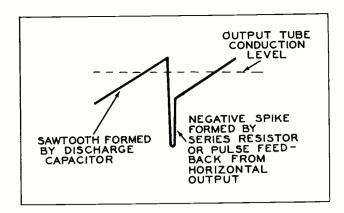
Figure 6. Horizontal Output Grid Waveform.
