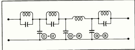
Figure 7. The Filter Network of Figure 6 in More Compact Form.
