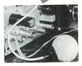
Figure 2. Safety Ball with Anode Lead Clipped in Place.
