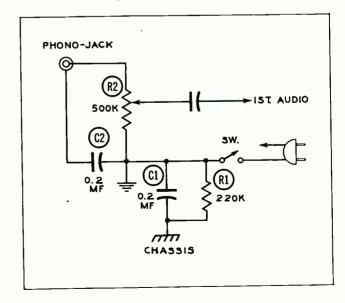
Figure 10. Phono-Jack; Low Side Through Capacitor to Floating Ground.
