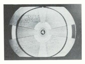
Figure 2. Diagonal Line Interference.
