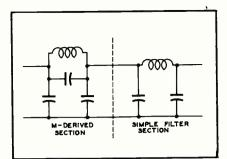
Figure 5. Combined M-Derived and Simple Filter Sections.
