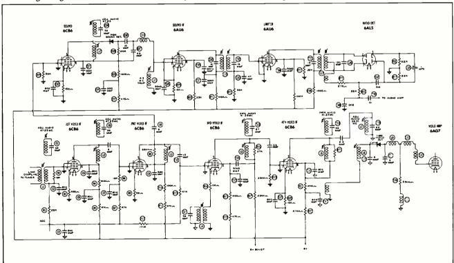
Figure 1. Partial Schematic of General Electric Model 24C10 Showing Sound Take-off Circuit.
