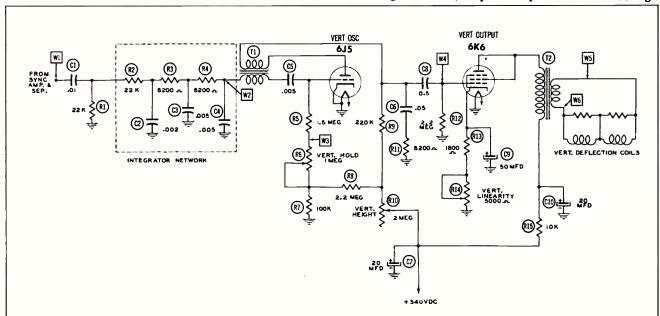
Figure 1. Typical Vertical Sweep System.
