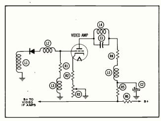
Figure 4-13. Variable Plate Supply Video Amplifier.
