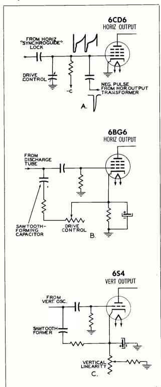
Figure 5. Typical Drive Circuits.
