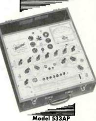
Larger, easy-to-read meter scale and a calibrated GM circuit provide increased accuracy in testing today's newer tubes.
