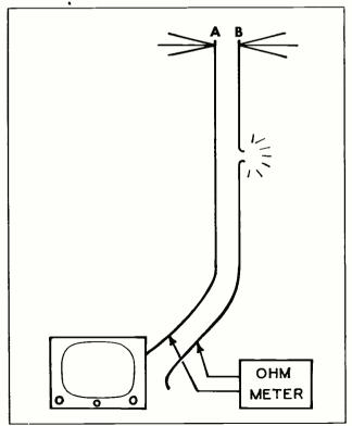
Figure 4. Setup for Checking an Antenna with an Ohmmeter.
