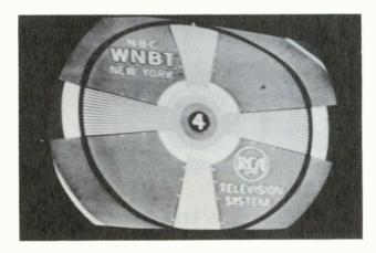
Figure 3. Linearity Affected by Presence of Undesired Magnetic Field.
