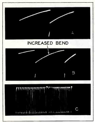
Figure 5. Waveforms at Point W4. (A) Normal. (B) With Leaky Capacitor C6. (C) With Open Capacitor C6.
