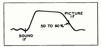
Figure 1. Picture Carrier IF Should Be at Least on the 50% Point of Slope.
