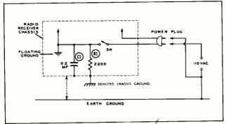
Figure 7. Floating Ground in an AC-DC Receiver.
