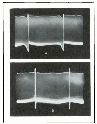
Figure 2. Waveforms at Point W1. (A) Normal. (B) With Inoperative Blocking Oscillator.
