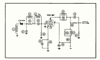
Figure 4-11. Single Stage Direct-Coupled Amplifier.
