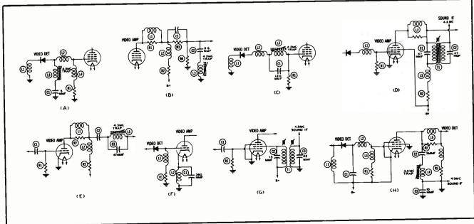
Figure 4-15. (A-H) 4.5 mc Trap Circuits.
