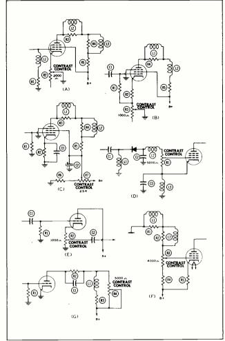
Figure 4-14. (A-G) Various Types of Contrast Control Circuits.
