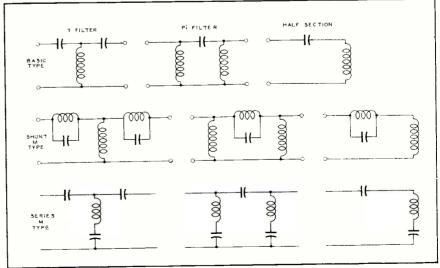
Figure 3. Three Classes of High-Pass Filters: T, Pi, Half Sections. Low-Pass Filters also Fall Into These Three Classes.
