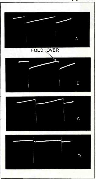
Figure 6. Waveforms Across Vertical Deflection Coils. (A) Normal. (B) With Leaky Capacitor C8. (C) With too Great a Decoupling Resistor R15. (D) With Open Capacitor C9.
