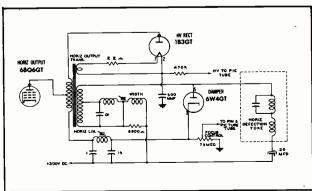
Figure 2. Low Voltage Focus Control Circuit.
