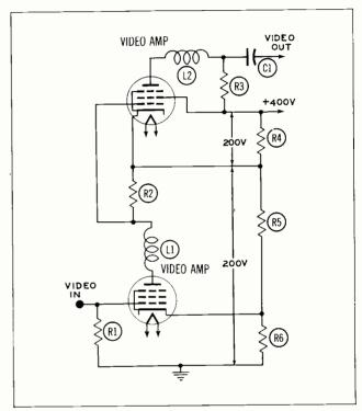
Figure 4-10. Simplified Schematic of Direct-Coupled Amplifier.
