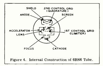
stream of electrons that are guided or focused toward the anode or plate. In the path of the electron stream is a limiter or first grid and a quadrature or second grid. These grids act as gates in the electron path. Either grid can cut off the electron stream.
