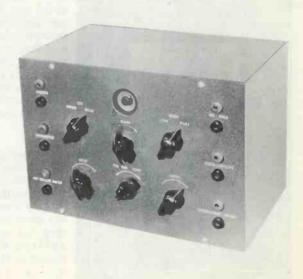
Figure 9. Completed view of Impedance Measuring Device with Null Indicator.
