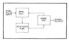
Figure 1. Block Diagram of the Stages in a Reactance Tube AFC System.
