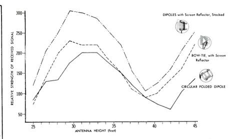
Figure 4. Relative Strength of Received Signal Versus Antenna Height at Position P-1 (1 Mile).
