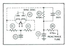
Figure 5. Between the Sync Discriminator and the Reactance Tube, There Is a Noise Immunity Circuit.
