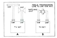
Figure 6. Methods for Connecting Transmission Lines to VHF-UHF Receivers.
