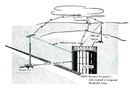
Figure 5. Sketch of the Terrain of Positions P-2 (3 Miles) and P-3 (3-1/2 Miles).
