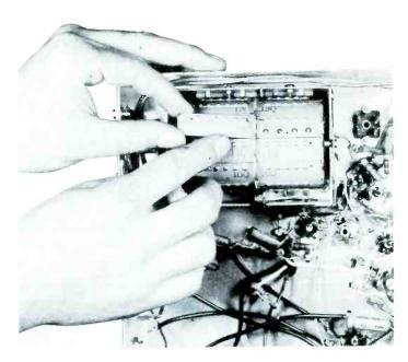
Figure 9. Installing the UHF Cscillator-Converter Strip.
