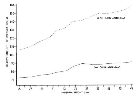
Figure 8. Graph of the Effect of Height on High Gain Antennas and Low Gain Antennas.
