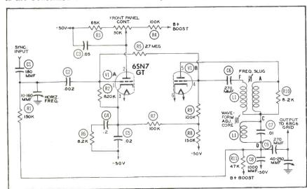
Figure 7. Schematic Diagram of a Pulse-Width AFC Circuit.
