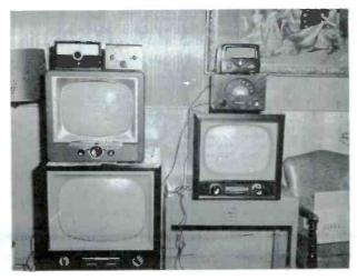
Figure 3. Some of the Converters and Receivers Employed During Tests.
