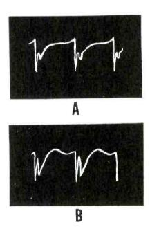
Figure 9. Other Waveforms of Importance in the Pulse Width System. (A) Grid of V1B, Figure 7. (B) Plate of V1B, Figure 7.
