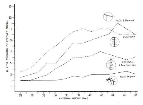
Figure 17. Graph of the Results Obtained at Test Positions F-5 (37 Miles) Using Four Different Types of Antennas.
