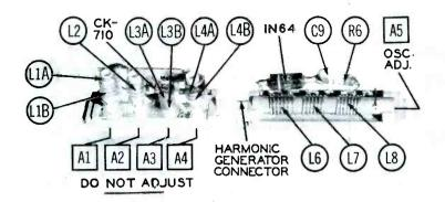
Figure 6. "34Q" UHF Strips Showing Component Placement.
