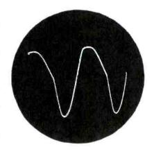
Figure 3. Waveform Which Is Present at Points A and B of Figure 2. Antenna Disconnected from Receiver.
