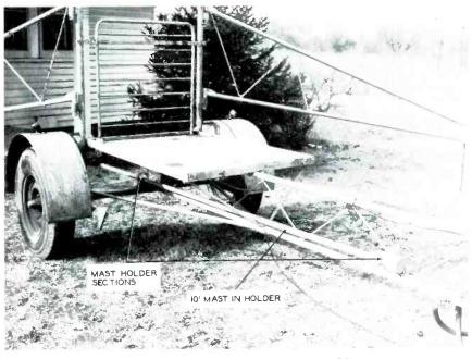
Figure 5. 10-Foot Length of Mast in Holders.
