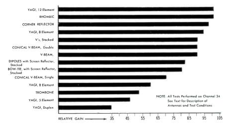
Figure 9. A Bar Graph Showing the Comparative Gains of the Various Antennas Tested at Position S-1 (20 Miles).
