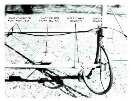
Figure 4. Mast Holder and Safety Chains.
