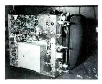
Figure 3. Bottom Chassis View of Motorola Receiver With UHF Converter Installed.
