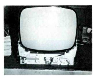
Figure 4. Front Chassis View of Motorola Receiver Showing Completed UHF Converter Kit Installation.
