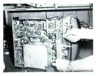
Figure 2. Placing the Motorola UHF Converter in the TV Chassis.
