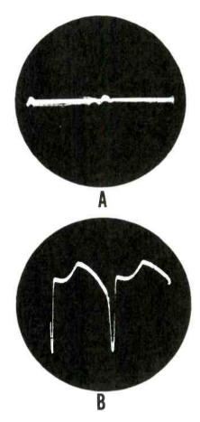
Figure 6. (A) Waveform at Grid of Reactance Tube When Noise Immunity Circuit Is Performing Properly. (B) Waveform Indication When Noise Immunity Circuit is Defective.
