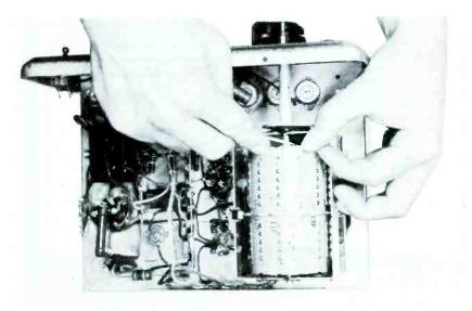
Figure 11. Installing UHF Strips in a Simpson 488 Field Strength Meter.
