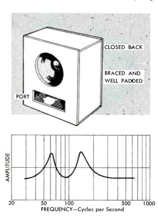
Figure 3. Reflex Enclosure With Impedance Curve.
