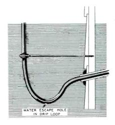
Figure 8. "Drip-Loop" With Condensation Escape Hole in Line.
