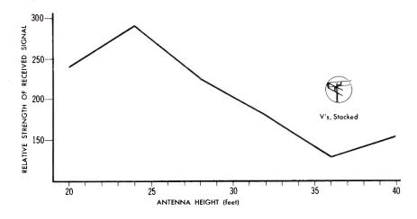
Figure 7. Relative Strength of Received Signal Versus Antenna Height at Position P-4 (5 Miles).
