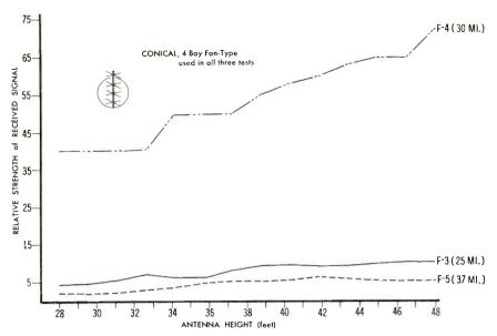
Figure 14. Graph of the Results Obtained Using the 4-Bay Fan-Type Conical at Positions F-3 (25 Miles), F-4 (30 Miles), and F-5 (37 Miles).
