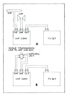
Figure 7. Common or Separate Transmission Lines Connected to Separate UHF Converter and TV Set.
