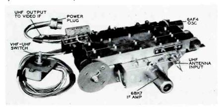
Figure 6. Front View of Raytheon UHF Converter Kit.
