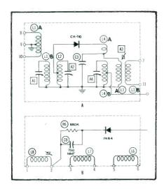
Figure 1. Schematic of Standard Coil UHF Strips. (a) Antenna Strip. (b) Oscillator Converter Strip.
