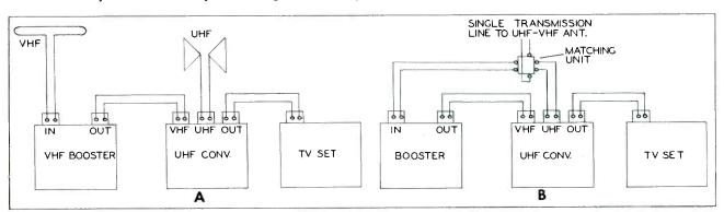
Figure 8. Connections for Common or Separate Transmission Lines to a Combination of Booster, UHF Converter, and Receiver.
