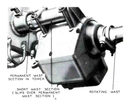
Figure 6. Rotator with Mast Sections in Place.
