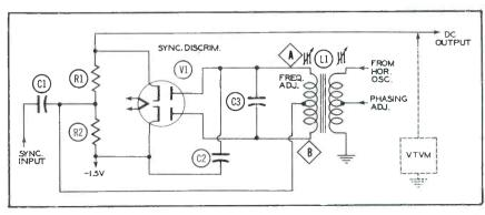
Figure 2. Simplified Circuit Diagram of the Sync Discriminator. A VTVM Should Be Connected as Shown to Check the Operation of the Circuit.
