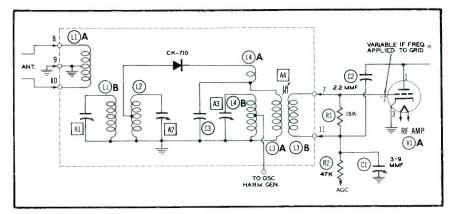
Figure 5. UHF Input Circuit.
