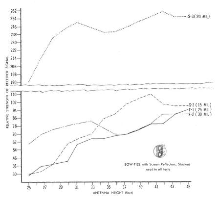
Figure 11. Graph Showing the Results Received Using the Stacked Bow-Tie with Screen Reflector at Positions S-2 (15 Miles), S-3 (20 Miles), F-1 (25 Miles), and F-2 (30 Miles).
