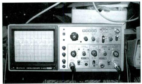
Figure 1. Check the drive waveform at the horizontal output transistor to determine if the horizontal circuits are functioning.
