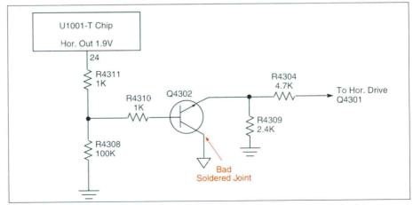
Figure 2. A poorly soldered connection on the collector terminal of Q4302 caused a dead-nostart-up symptom.
