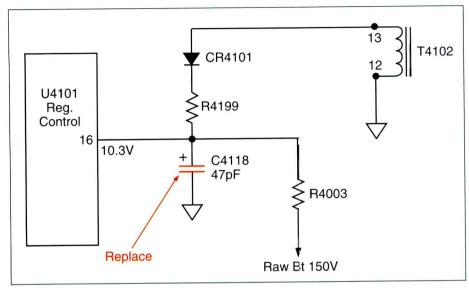
Figure 6. Electrolytic capacitor C4118 (47uF) connected to the regulator control IC caused the intermittent start-up problem in a RCA CTC169 chassis.
