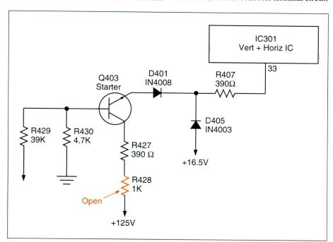
Figure 3. Replacing open R428 (1K) ohm resistor corrected a complaint of no start up in a Samsung CT5002DA TV.
