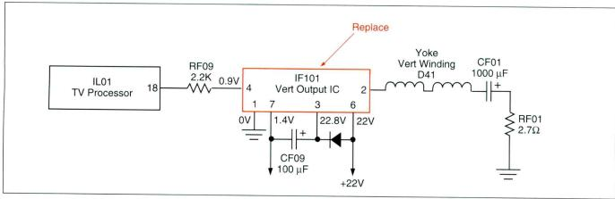
Figure 8. A leaky vertical output IC (1F01) caused an intermittent startup within a RCA TX81 chassis.
