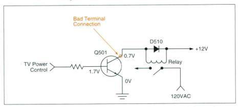
Figure 2. A bad soldered connection of relay driver transistor collector terminal caused an intermittent-dead Emerson VT1920 TV/VCR.
