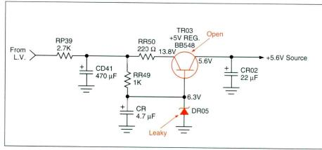
Figure 4. Replacing the +5V regulator transistor in a RCA TX82 chassis solved the intermittent start-up problem.
