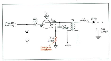
Figure 7. Resistor R16 (0.15ohm) in the drain terminal increased in resistance producing intermittent start-up.
