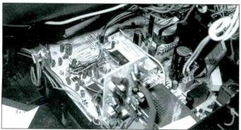
Figure 5. Resolder the control micro IC terminals to solve the slow turnon symptom in a RCA CTC177 chassis.
