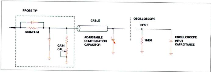
Figure 5. A high-voltage probe for an oscilloscope is really a relatively uncomplicated device: a properly insulated body containing a probe, a voltage divider \, and an oscilloscope probe lead.
