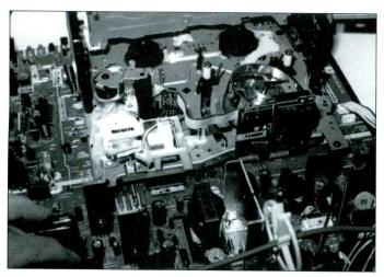
**Figure 3.** Use the negative terminal of the largest filter capacitor in the power supply as the "hot" ground terminal for voltage measurements.
