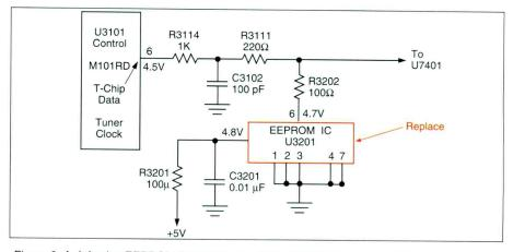
Figure 9. A defective EEPROM (U3201) in the RCA CTC177 chassis made the chassis cycle on and off.
