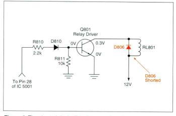
Figure 4. The shorted diode (D806) across the relay prevented a click or turn on of relay RL801 in a Panasonic TV/VCR.
