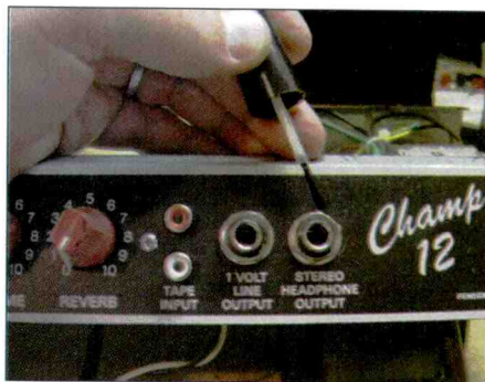
Figure 5. A bit of clear nail polish should lock these nuts in place preventing future problems.
