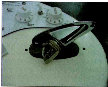
Figure 12. Removal of the output jack plate to get to the jack. Note that this particular guitar has midi circuitry, requiring a jack that cuts out this circuit whenever a plug is inserted.
