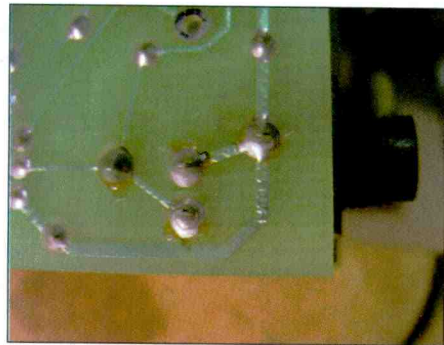
Figure 6. Even with all the obvious physical damage, here is the main reason the amp was brought in for repair: intermittent sound because of CSJs.
