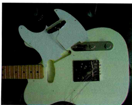
Figure 17. This is a Tele with pickguard lifted. With only two pickups, one attached to the pickguard, a “Tele” is about as simple as an electric guitar can get.
