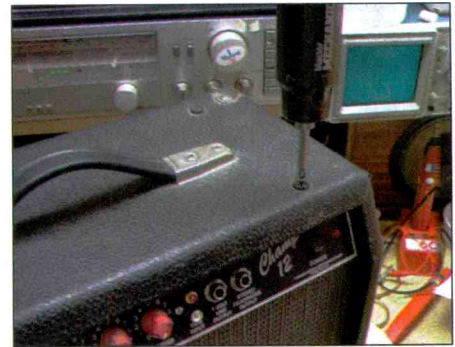
Figure 7. Generally, the screws holding the chassis in place are on top of the cabinet.
