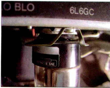
Figure 11. Most tubes hang upside down, and are held in place by metal retainers. Tube removal is a two-handed operation.
