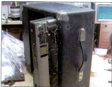
Figure 4. The chassis partially removed from the cabinet. Note the amp was turned on its side to aid removal.
