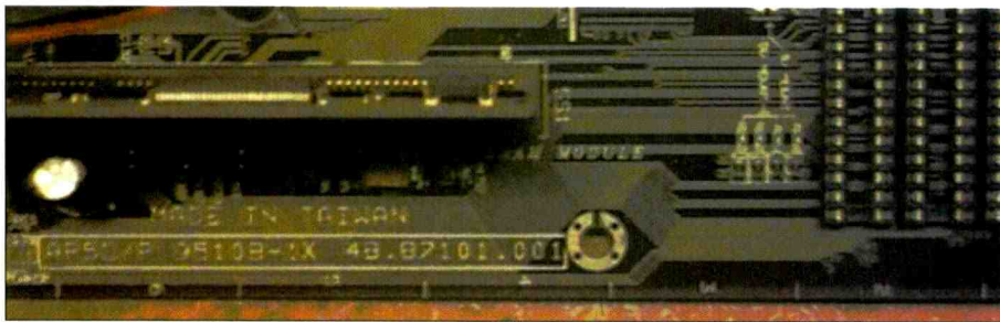
Figure 1D. Board ID on edge of board, near cache slot.
