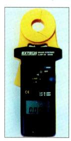
autoranging mA and resistance measurements. Ground Resistance measurements range up to 1500W with 0.01W resolution. Leakage current to 15A can be measured with 0.001 m A maximum resolution.
