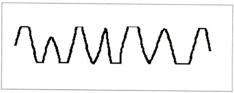
Figure 2. If we take the same music as that represented in Figure 1 and try to reproduce it at a level greater than the amplifier is capable of (clipping), we get something like this waveform, which looks more like a group of square waves than a sinusoid. Square waves contain large amounts of high frequency information, which can destroy tweeters.
