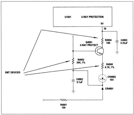
Figure 4. Critical SMT resistor chips are also located in the X-Ray protection circuits of an RCA CTC187 chassis.
