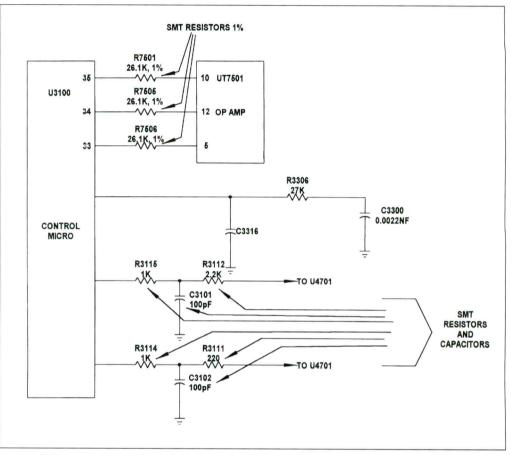
Figure 1. These are some of the critical SMT resistor chips found in the system control circuits.
