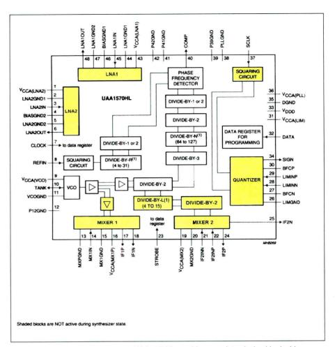
Figure 3. The Philips Semiconductor UAA1570HL provides complete single-chip double-superheterodyne receiver front-end that operates with signals from GPS and GLONASS navigation systems. The IC integrates a programmable DPLL synthesizer, VCO with external varactor and resonator, a 1-bit amplitude quantizer and a time sampled TTL/CMOS compatible SIGN output bit driver.
