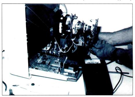
Figure 5. Making a continuity test of a normal fuse with the ESR meter.
