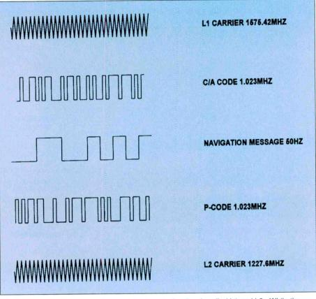
Figure 1. The satellites transmit two microwave carrier signals called L1 and L2. While the 1575.42 MHz L1 signal carries the navigation message and the SPS code signals, the 1227.60 MHz L2 frequency measures ionospheric delay.
