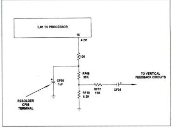
foil trace and PC **Figure 9.** A faulty soldered terminal of CF08 produced insufficient vertical wiring. The ESR sweep symptom in the RCA TX82 chassis.
