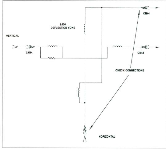
Figure 6. Improperly soldered connections of CN44 caused horizontal foldover in a Samsung K20 chassis.
