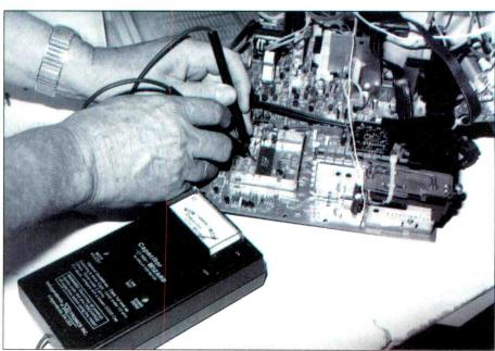
**Figure 7.** Check each pin terminal of IC or microprocessor with the ESR meter to insure a good soldered connection.
