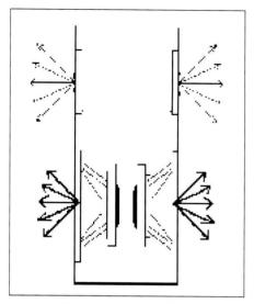
Figure 3. The front and back drivers in a bipolar speaker move at the same time with the music. These speakers are used as the main speakers in stereo and the front right/left speakers in a home theater system. The front output sound provides direct information that is crucial to detail, focus and localization.
