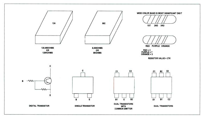
Figure 3. The values of SMD capacitors and resistor chips are marked on top with numbers and letters.
