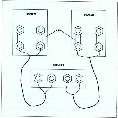
Figure 5. Speakers designed so that they can be connected in a bi-wire arrangement come from the factory with a connecting link between the terminals so they can be wired normally, as shown here
