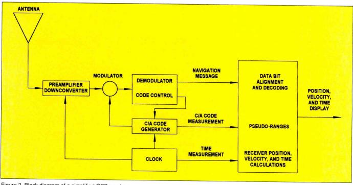
Figure 2. Block diagram of a simplified GPS receiver.
