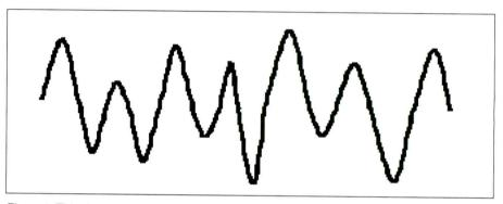
Figure 1. This sinusoidal signal represents what an audio signal might look like as it enters the speaker.
