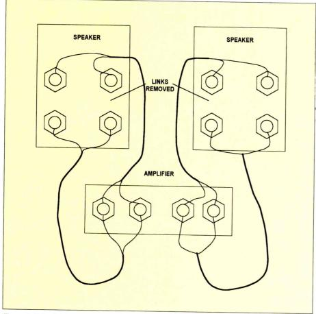
Figure 6. If the link between corresponding terminals of a bi-wire type speaker is removed, the speaker can be bi-wired
