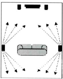
Figure 4. Dipolar speakers have come into existence primarily within the home theater realm, where they are generally located directly on the sides of the listener. Since the front and back of this speaker are out of phase with each other, the surround speaker has a null or cancellation zone within the movie viewing area. Thus, the focus of sound transcends forward to the movie screen with the surround speakers enveloping the listening area.
