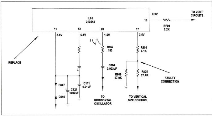
Figure 8. Faulty soldered connections of RP03 and RP05 caused poor vertical sweep in a RCA TX82 chassis.
