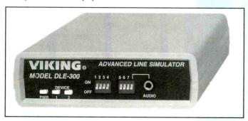
The simulator also provides instant point-to-point communication with ring-down notification. As soon as one connected phone goes off-hook, it immediately rings the other phone.
