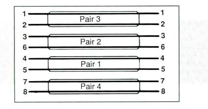
Figure 8. Wiremapping simply means that each wire is hooked up correctly, with no open wires or shorts. Most wiremapping failures are simple enough to understand, like reversed wires in a pair, crossed pairs or opens and shorts. The most difficult wiremap problem is a split pair, when one wire on each pair is reversed on both ends.
