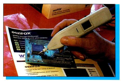
This oscilloscope is small enough to fit in a technician's pocket, and provides a 5Mhz bandwidth.
