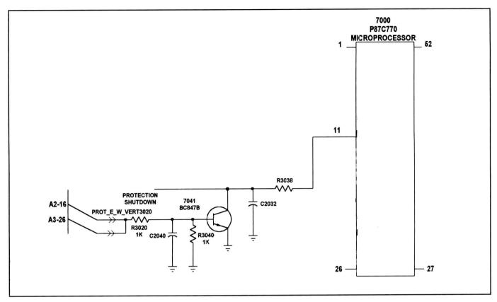
Figure 4. If vertical deflection in this set is lost, transistor 7716 turns off, permitting transistor 7041 to turn on and pull pin 11 of IC 7000 low. When pin 11 goes low, the microprocessor "assumes" that vertical deflection has failed and responds by turning the TV off.
