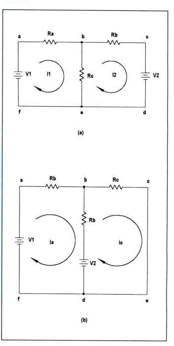
**Figure 1.** If you are going to use Maxwell's loop equations in Figure 1(a) to solve for the current through  $R_{\rm C}$ , you must first solve for  $I_1$  and  $I_2$ . Then you must subtract those currents to get the value of  $I_{\rm C}$ . However, if you move branch b to the outside, as shown in Figure 1(b), you only need to solve for one current ( $I_{\rm C}$ ) to get the current ( $I_{\rm C}$ )through  $R_{\rm C}$ .
