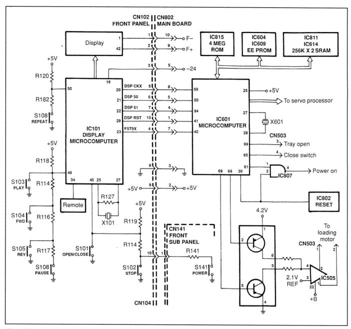
Figure 5. System control monitors and directs all functions of the DVD 400/420. The circuit includes the main microcomputer (IC601), the SRAM (IC611 and IC614), the EEPROM (IC604 and IC609), and the four meg ROM (IC615).
