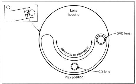
**Figure 2.** Some DVD players utilize two optical pickups, one to play audio CDs and another to play DVDs. The Magnavox player uses one optical block equipped with two lenses to achieve the same purpose.
