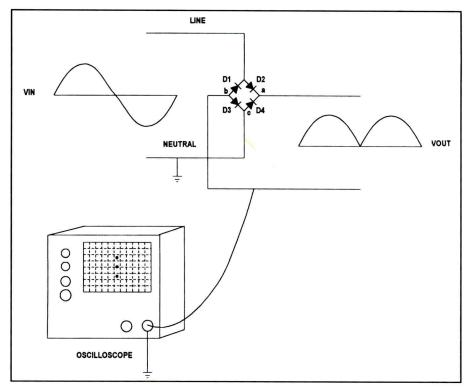
**Figure 3.** When you use an oscilloscope to check what's going on in the hot part of a chassis that features a full-wave bridge rectifier, you connect the grounded negative probe to the chassis hot ground. Now when you turn the unit on, as before, D1 is forward biased with the entire Vmax across it and it is destroyed.
