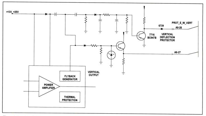
Figure 3. Transistor Q7716 provides vertical deflection protection in this set.
