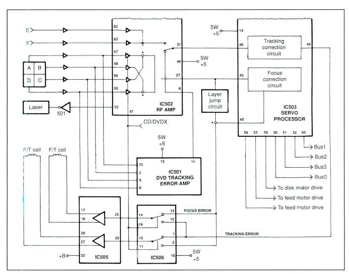
Figure 1. The laser, which functions as a single beam system for the DVD disk and as a three-beam system for the audio disk, and the laser pick-up, develops the signal that the servo system uses to control focus and tracking.
