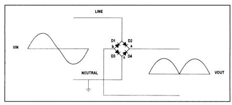
**Figure 1**. A full-wave bridge rectifier effectively inverts the negative-going segment of the power line ac. Note that the common side of the rectifier's output is not grounded.
