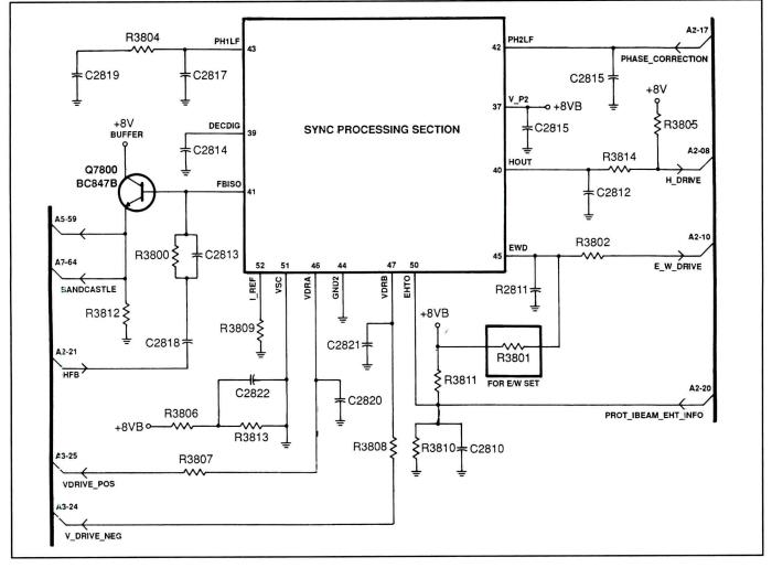
Figure 2. The voltage at pin 50 of IC 7150 should be about 0.8V when the TV is in standby, about 2.2V when the TV is on and not receiving a signal, and about 2.5V when it is on and receiving a signal.
