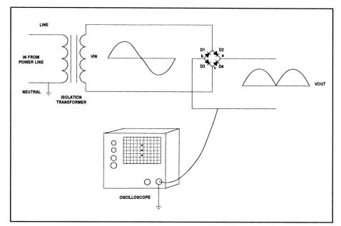
**Figure 4.** When you connect the set to the power line via an isolation transformer the output of the transformer is the 120V line voltage, but neither output line is grounded. Point c is no longer at ground potential, and now the technician can safely connect the grounded oscilloscope probe to point b.
