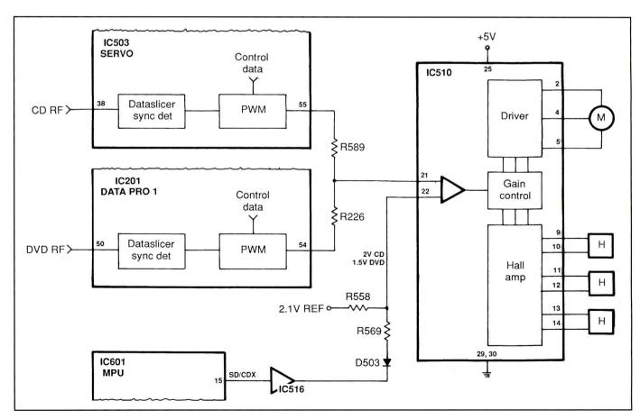
Figure 3. When a DVD disk is inserted into the player, after focus has been achieved, the pickup begins to generate an RF signal which is applied to pin 50 of IC201, the so-called "data processor one."
