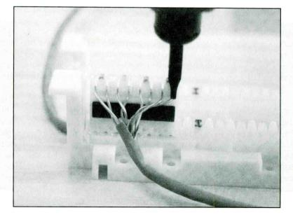
Figure 3. A 110 punchdown block. This type of connecting block is most popular for LANs.
