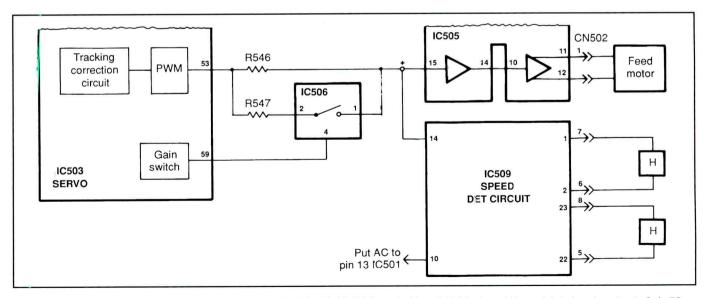
Figure 4. Feed motor drive from the tracking correction circuit inside IC503 is routed to a PWM (pulse width modulator) and sent out of pin 53 on its way to pin 15 of IC505, the feed motor drive IC. If you are watching a DVD, the drive goes through R546 before it reaches IC505. If the disk needs to be speeded up, the gain switch inside IC503 turns on IC508 switching R547 in parallel with R546 to increase the gain of the signal.
