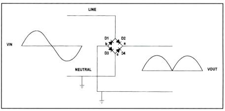
**Figure 2.** If point b were grounded, in effect diode D3 would have a short circuit placed across it, as both ends are at ground potential. Now when the line voltage goes negative the voltage forward biases D1, effectively placing the entire Vmax across that diode.
