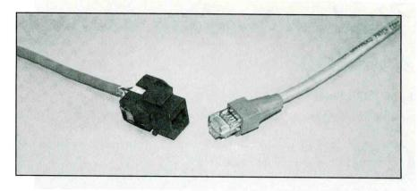
Figure 2. RJ45 is the popular name of the modular 8 pin connector used with UTP cable in structured cabling systems.
