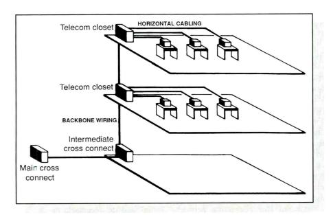
Figure 5. The telecom cable industry has developed terminology for the areas where cable connections are made and the runs between those locations.
