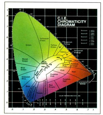
**Figure 9.** A chromaticity diagram graphically depicts the relationship between hue (light wavelengths) and purity and allows the specification of individual colors with an x-y grid system.
