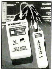
10Base2 cable (coax) and RJ45/RJ11 modular cables, TIA-TIA-568B, 568A, and Token Ring cables by comparing one transmitting end to the corresponding receiving end. It tests point-to-point rather than pair-to-pair. By utilizing the supplied remote kit, the Model 231 can test cables installed as far away as 1,000 feet, either on a wall plate or patch panel.
