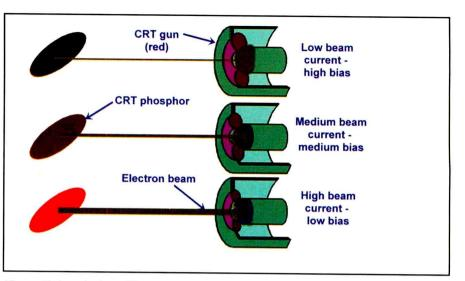
**Figure 13.** In order for a CRT to produce an image on the screen, the intensity of the electron beam from the cathode to the phosphor screen must be made to vary. Changing the bias voltage in step with the video image to be produced varies the beam current. White and bright colors require high beam current, while grays and dark colors require a small beam current.
