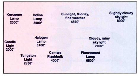
**Figure 11.** Common light sources range from a color temperature of around  $2500^{\circ}$  K (more red) to over  $9000^{\circ}$  K (more blue). Equal energy white is approximately  $6000^{\circ}$  K.
