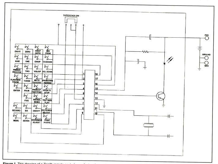
Figure 1. This drawing of a Zenith remote control manufactured sometime between 1985 and 1995 shows the functioning of a typical handheld unit. If any of the push-button switches are dirty, the unit won't send the correct signal to the receiving unit in the TV set or VCR.
