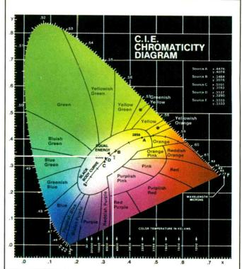
**Figure 10.** The C.I.E. diagram provides a grid coordinate system to specify a precise measurement of any spectral color or color combination. A C.I.E. coordinate of x=0.333 and y=0.333, specifies the white light perception produced by equal light energy of all wavelengths.
