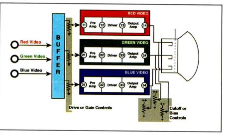
Figure 14. Video display circuits include two sets of adjustments to produce neutral white and proper grays and colors over the entire brightness range.
