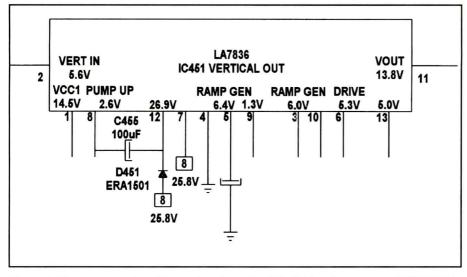
Figure 2. There was no sign of B+ at pins 7 and 12 of IC 451 in a Quasar model TS2523EK, which exhibited the symptom of failure of the vertical deflection.
