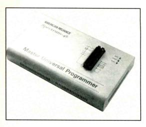
ating environment. With an onboard processor and Field Programmable Gate Array (FPGA), the 48-pin driver system provides the means of handling numerous DIP-style silicon PLD's, microprocessor, and high-density memory chips.
