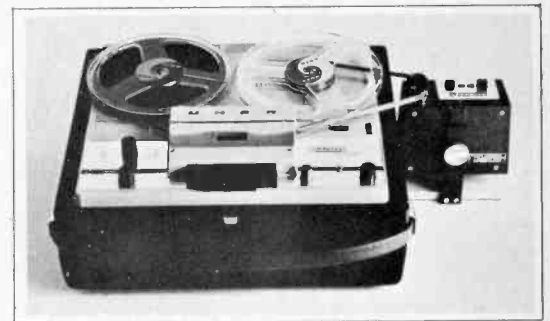
Its unusual "Dia-pilot," the impulse transmitter that automatically synchronizes and controls slide projections is a popular feature of the UHER 6000 portable.
