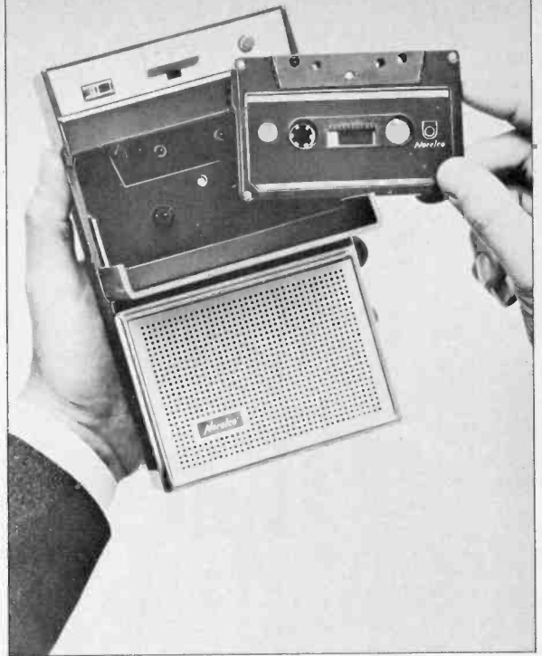
The "Carry-Corder" by Norelco is a portable, cordless, cartridge-fed fully transistorized tape recorder.
