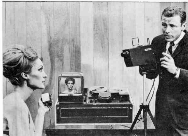
Sony's new home video tape recorder shown with camera, microphone and monitor.
