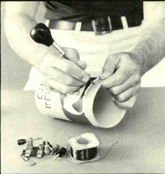
2. Punch four holes in the box, vertically aligned, two at the top and two at the bottom. (Give it your awl.)
