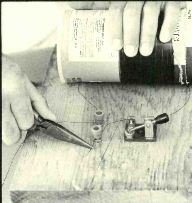
6. Join the previously unattached crystal terminal to the other binding post with a short piece of wire.
