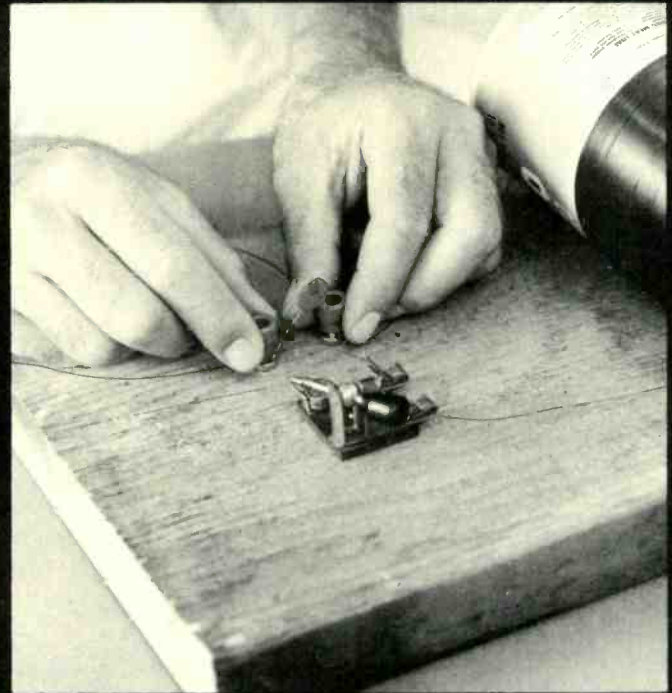
7. Place the capacitor between the two binding posts.
