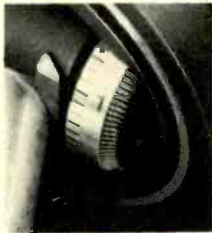
Stylus pressure dial calibrated in tenths of a gram from 0 to 1.5 grams; in quarters of a gram from 1.5 to 3.0 grams.
