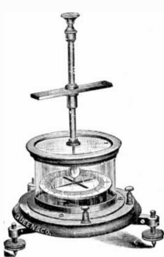
FIG. 1,287.—Queen reflecting astatic galvanometer. It is mounted on a mahogany base with leveling screws. A plain mirror is attached above the upper needle. The entire combination of mirror and needles is suspended by unspun silk from the interior of a brass tube, which also carries a weak controlling magnet. A dial 4 inches in diameter and graduated in degrees, enables the deflections of the needle to be accurately read. The mirror can be used with a reading telescope and scale, or by means of a lantern, the image of a slit may be reflected from the mirror to a screen. Resistance, .5 to 1,000 ohms.
