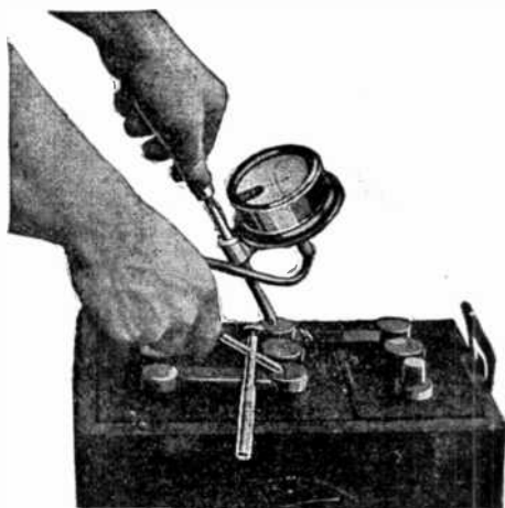
FIG. 1,737.—Combination cell tester for open voltage and cadmium tests. It does away with separate meter and prods. Cadmium extension removable for immersion when not in use.
