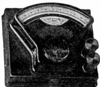
FIG. 1.345.—Weston portable standard ammeter with self-contained shunts. The pointer is knife edged and each instrument is equipped with a zero correcting device.
