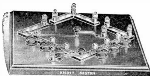
FIG. 1,488.—Knott demonstration Wheatstone bridge, diamond form for practical application of Wheatstone diagram in determining resistance. As will be noted from the illustration, all connections and coils are mounted on a base according to the Wheatstone diagram as found in standard text books. In the "ratio arms" are coils of 1, 10 and 100 ohms. The "balance arms" are provided with gaps each with non-detachable binding posts, one pair for the "known" and one pair for the "unknown" resistance. Binding posts and a key are provided for the battery and galvanometer circuits.
