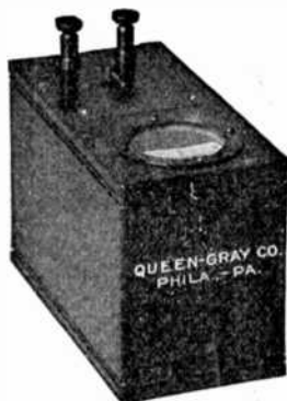
FIG. 1,328.—Queen portable D'Arsonval galvanometer. The deflections are proportional to the current and the scale has 30 divisions each side of the center. A zero adjustment is provided.
