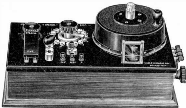
FIG. 1,539.—Leeds and Northrup Type K Potentiometer. It has no internal resistance which gives high sensitivity. There are no contact resistances in the potentiometer circuit proper. The last one tenth volt is covered by a slide wire which facilitates following a fluctuating voltage. The current flowing through the potentiometer may be checked without disturbing the dial or slide wire setting. When used with any cadmium cell the potentiometer is direct reading, requiring neither calculations nor corrections. The construction of the instrument is further shown in the diagram fig. 1,540.
