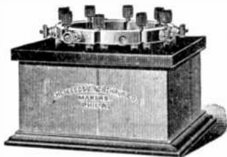
FIG. 1,475.—Leeds and Northrup Standard high resistance box, 100,000 ohms equipped with short circuiting switch. When the switch is thrown to the right the box is short circuited and when thrown to the left the resistance of 100,000 ohms is placed in the circuit.
