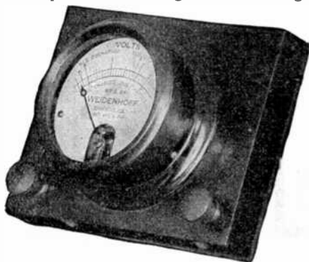
FIG. 1,703.—Weidenhoff cadmium test meter. Designed to give the open voltage of a cell and the reading positive and negative plates to cadmium.
