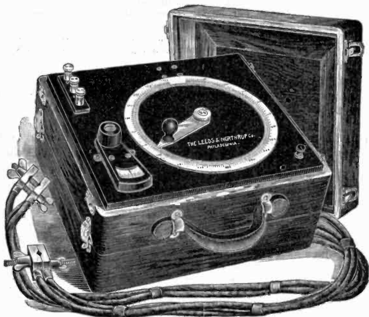
FIG. 1,564.—Leeds and Northrup bridge for locating faults in power circuits. From the diagram of connections shown in fig. 1,565, it will be seen that the instrument operates on the slide wire principle. A galvanometer is mounted in the instrument, and the necessary leads for connecting to the cable under test are provided. Fault locations are made by means of the Murray loop test. Mounted upon a circular block inside the case of the instrument is a low resistance slide wire. This wire is made large so that a heavy test current may be used, thus giving a good sensitivity in making locations. A sliding contact moves upon the bridge wire, and carries with it a pointer moving over a scale on the top of the containing case. This scale is divided into 980 divisions, each division being about two millimeters. The graduations on the slide wire dial stop ten divisions either side of the ends. The end divisions are marked 10 and 990. The resistance of each lead is therefore equal to the resistance corresponding to ten divisions of the slide wire. It will thus be seen that the slide wire actually begins at the outer end of the leads, thus entirely eliminating lead resistances.
