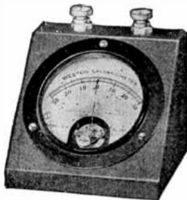
FIG. 1,305.—Weston portable student galvanometer. Resistance approximately 25 ohms. The current required for a millimeter (one scale division) deflection is 22 micro-amperes. With 1 volt, a deflection of 1 millimeter will be obtained through 45,500 ohms, but as a deflection of .2 of a millimeter can be readily detected, the galvanometer is, in reality, serviceable through 227,500 ohms. This galvanometer is designed for the use of students in colleges and schools, for making bridge measurements, and for the detection of small currents.
