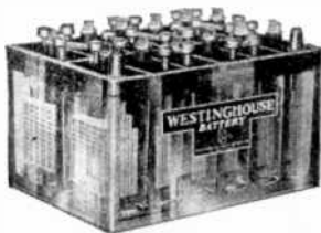
FIG. 1,591.—Westinghouse 12 compartment glass case radio storage B battery. 24 volts; capacity 3,500 milliamperc hours (3.5 ampere hours) when discharged at a rate of 40 milliamperes. The clear glass case gives the user a view of the action of the battery on charge and discharge, and permits a ready inspection of plates and separators as well as the level of the acid solution. A layer of sealing compound over the rubber covers and around the posts keeps this battery free from acid leakage.
