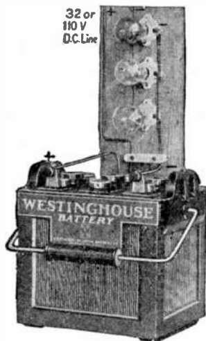
FIG. 1,893.—Set up showing connections for charging 2 B batteries in series from a 110 volt direct current line. The lamp is shown in the negative lead but may be connected in either lead. Not over 3 batteries may be charged in series from a 110 volt line.
