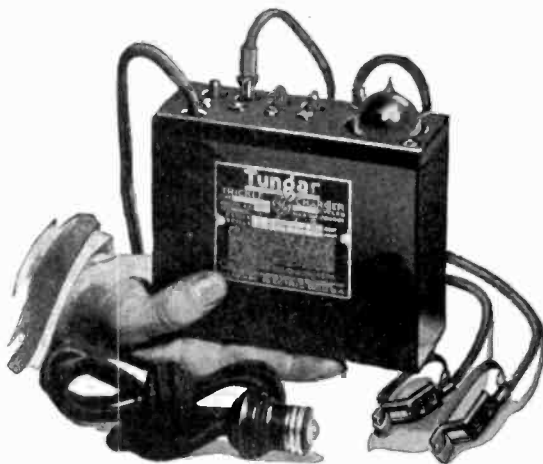
FIG. 1,724 —Trickle charge. When a number of batteries are to be held in wet storage, the most satisfactory results can be obtained by charging continuously at a very low rate, which is so low that gassing is avoided and yet gives enough charge, to maintain the batteries in good condition. This charge is called a trickle charge and in many cases will be found more convenient to arrange for than the periodic charge. It has the added advantage of keeping the batteries in condition for putting into use at any time on short notice. To apply trickle charge: 1, give bench charge; 2, Connect a tungsten lamp or lamps of appropriate resistance, in series with the cells, across a charging system adapted for continuous charging. 3, Every two months interrupt the trickle charge, remove filling plug, add water to bottom of filling tubes,
