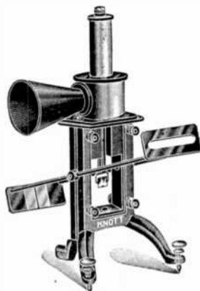
FIG. 1,322.—Knott radio micrometer heat indicator. It contains the fundamental parts of the D'Arsonval galvanometer, but with the moving coil replaced by a sensitive thermoelectric couple. A candle flame 50 ft. distant will cause a marked deflection. The deflecting horn is mounted on a movable ring, so that the heat can be received from either side only. The heat from the body of the observer therefore cannot affect the readings.
