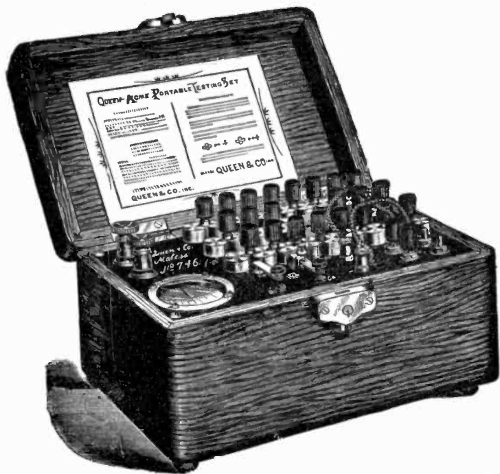
FIG. 1,501. —Queen Acme portable testing set. It consists of a Wheatstone bridge, with reversible arms, battery of four dry cells, D'Arsonval galvanometer, battery and galvanometer keys. There are sixteen resistance coils, having a combined resistance of 11,110 ohms. Each bridge arm is provided with three coils of 1, 10, 100 ohms, and 10, 100, 1,000 ohms respectively. The commutator admits of a ratio of 1 to 1,000 on either bridge arm, giving the set a theoretical range from .001 of an ohm to 11,110,000 ohms. For resistances above 1,000,000 ohms, the normal battery power must be increased. The contact keys are located as shown. The battery key has single contact, but the galvanometer key has double contact; depressing it closes the galvanometer circuit, and releasing it short circuits the galvanometer, bringing the latter quickly to rest.
