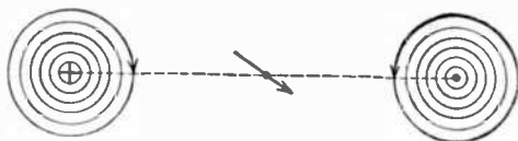
FIG. 1,290.—Horizontal section through middle of tangent galvanometer, showing magnetic whirls around the coil and corresponding deflection of needle.
