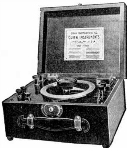
FIG. 1,535.—Queen ground resistance and direct reading ohm meter for measuring the resistance of ground connections and driven grounds. This tester although direct reading is arranged on the Wheatstone bridge principle, thereby giving a uniform scale with maximum accuracy throughout its entire range. It is balanced by a telephone receiver. The use of the bridge rheostat in the form of a slide permits measurements to be made with facility and speed. The method of use is the "three ground test" which requires the determination of the combined resistance of the ground under investigation and of two auxiliary grounds which are connected in series with it and with each other. To increase the range of this tester, a 10 multiplier in the bridge arms is provided, permitting its use as a general purpose ohm meter for ordinary resistance measurements, up to a maximum of 2,700 ohms. The direct scale reads from 0 to 270 ohms on one ohm divisions. The single scale division can be easily estimated to one half ohm. When the multiplier is in circuit the scale range is 0 to 2,700 ohms. Binding posts and switches are arranged so that an external galvanometer can be connected to the instrument, as some may prefer a galvanometer for balancing in place of the telephone when measuring ordinary resistances. When used for ground resistances a telephone is necessary.
