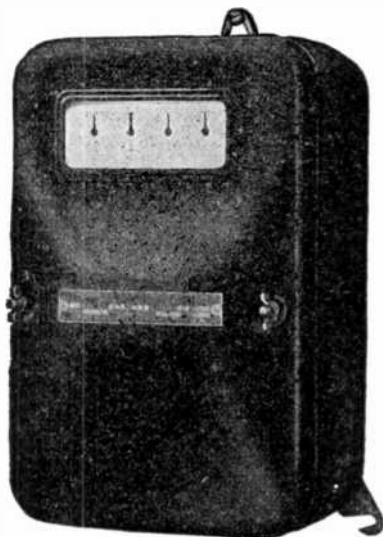
FIG. 1,381.—General Electric, Thomson type C-6 direct current watt hour meter. It is standard practice to furnish flexible cable leads provided with copper terminals for meters of 100 amperes capacity and above. For meters of lower capacity, the leading-in wires are fastened to suitable brass binding posts with set screws.
