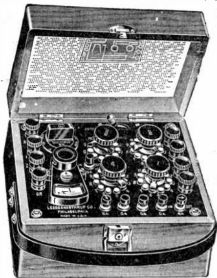
FIG. 1,519.—Leeds and Northrup type T, testing set. It is provided with the necessary connections for making resistance measurements, and for locating faults by the Murray and Varley loop methods. The addition of a simple buzzer and telephone receiver permits the location of opens as well as a single three-way switch, of the type used on telephone switchboards makes possible, with a single motion, immediate connections for resistance, or Murray loop, or Varley loop tests. The switch replaces the two single pole, double throw switches ordinarily used on testing sets. Provision is made for connection of an external battery and galvanometer in the relatively few instances where this may be necessary; and, without changing connections, either internal or external battery or galvanometer may be used. Protective resistances in both internal and external battery circuits guard against burn-outs or overheating of the adjusted coils in the set.
