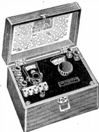
FIG. 1,506.—Leeds and Northrup ohm meter. It consists essentially of a slide wire Wheatstone bridge with the scale divided to read in per cent of a fixed resistance value. A galvanometer is mounted on the containing case of each battery and galvanometer keys are provided. These ohm meters, being slide wire bridges, the greatest accuracy is at the center of the scale. Fixed coils of 1, 10, 100, 1,000 and 10,000 ohms are contained in the instrument with a plug arrangement allowing any one to be used. When a balance is obtained the actual resistance is determined by multiplying the dial reading by the value of the fixed coil in use. This amounts simply to shifting the decimal point. For instance, if the 100 ohm coil were being used and the pointer were at .875, the resistance would be 87.5 ohms. Accuracy 1% over the range .3 ohm to 30,000 ohms.
