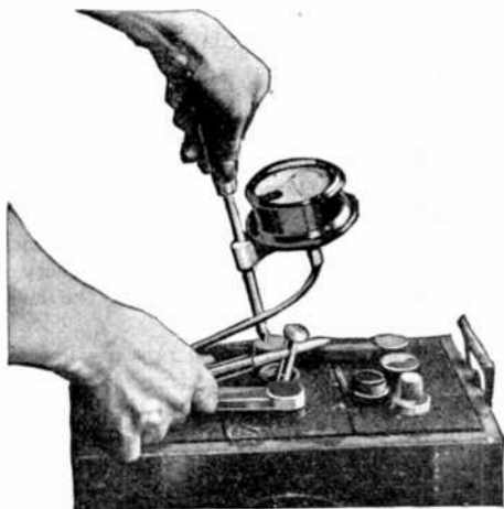
FIG. 1,704.—Weidenhoff cell tester: view showing operator taking open voltage cell reading. It is useful in checking the voltage of batteries while on the charging line.
