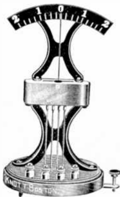
FIG. 1,282.—Knott lecture table galvanometer. Adapted for use in simple lecture table experiments, where high sensibility is not essential. The scale is large and open.
