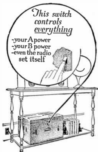
FIG. 1,855.—Philco AB socket power. It eliminates both A and B batteries. Filament current is supplied at 4 volts, thus protecting the delicate filaments of the dry cell tubes from over voltage. Plate current is supplied at either 90 or 130 volts or both as required by the new Radiola and other sets using UX-120 tubes in the last audio stage. The 130 volts are fixed. The 90 volts are adjustable, by means of a single knob, through a range of 60 to 100 volts.
