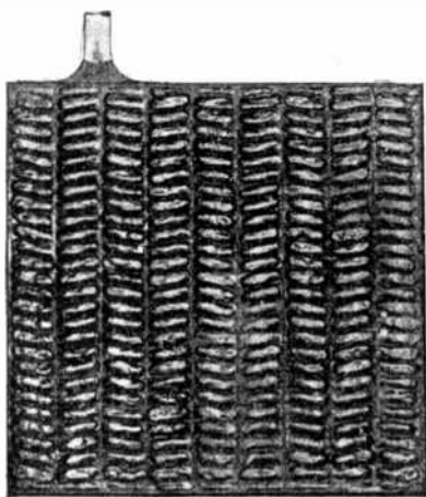
FIG. 1,684.—Battery under charged for long interval. If the battery had been under charged for some time (sufficiently long to allow the plates to become hard) and then over discharged, the additional lead sulphate formed during the over discharge would make room for itself by blowing out the little granular chips of active material, leaving the plate in a pitted condition as shown in fig. 1,683. Again, the additional lead sulphate from over discharging may make room for itself by buckling the plates or cracking the grids. Therefore, a pitted plate, a buckled plate or a cracked grid always indicate prolonged under charging followed by over discharging.
