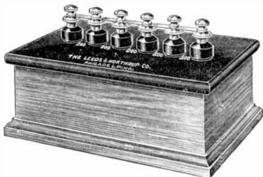
FIG. 1,474.—Megohm box or set of standard high resistances. The box contains five resistances of 200,000 ohms each. The six pillars are petticoat insulated, the resistances being placed between each pair of pillars. There is a double contact post on top of each pillar so that these can be connected together with copper links.
