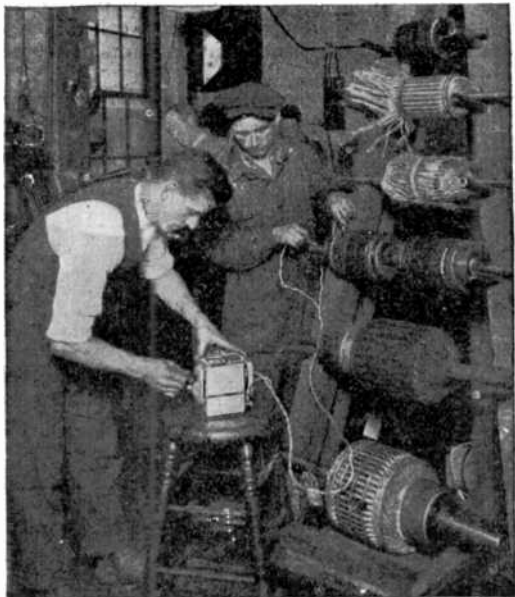
FIG. 1,573.—Testing armatures with Biddle "Meg" insulation tester in an electrical repair shop.
