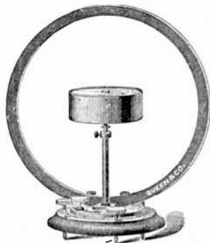
FIG. 1,299.—Queen tangent and sine galvanometer. This instrument properly adjusted can be used as a standard instrument for laboratory work. The brass ring is 12 inches in diameter, and the grooves in which the wire is wound are carefully turned so as to be of true rectangular cross section, thus allowing the constant of the instrument to be accurately calculated and compared with the constant as obtained by other methods. The compass box is 5 inches in diameter and is so held in position that it may be raised or lowered, rotated on its vertical axis, shifted out of the plane of the coil, etc., thus enabling the operator to acquire proficiency with the instrument and to meet all cases of derangement possible. The dial is graduated to single degrees, and the needle is suspended by a very light cocoon fibre. The whole instrument can be turned about its vertical axis, and a quadrant graduated in degrees upon the base allows the amount of rotation to be accurately measured, and the laws of the sine galvanometer investigated. The instrument is wound to measure .25 amperes to 8 amperes.
