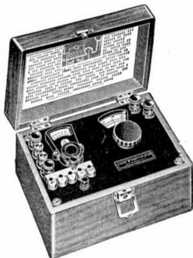
FIG. 1,525.—Kelvin bridge ohm meter for measuring low resistance. It is similar in construction to the familiar Wheatstone bridge type ohm meter. Accuracy: 2% between .0001 ohm and 11 ohms; Galvanometer: sensitivity 1. megohm, resistance 40 ohms; General: five ranges. Self contained No. 6 dry cell battery.
