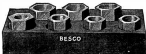
FIG. 1,741.—Post builders. When a battery is opened the posts of the plate straps must be drilled down and again built up on assemblage. There are seven necessary sizes, ranging from 3/8 to 1/4 in.
