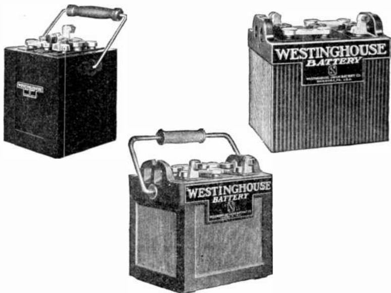
FIGS. 1,850 to 1,852.—Westinghouse storage A batteries. Fig. 1,850 is a 7 plate battery of 60 ampere hour capacity and is used on the smaller radio sets where the filament requirements are not so heavy as in the multiple tube sets. Fig. 1,851 is a nine plate 80 ampere hour battery equipped with terminal and thumb nuts. It is adapted for sets of any size where convenient arrangements have been made for recharging. Fig. 1,852 is an eleven plate battery having a capacity of 100 ampere hours at a 3 ampere intermittent discharge rate. Burned on terminals with thumb nuts, the positive and negative on the same side make it easy to attach to set.
