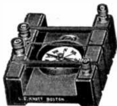
FIG. 1,278.—Knott galvanoscope. It has three separate circuits, 1, 25 and 100 turns with binding post for each circuit.
