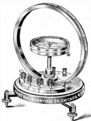
FIG. 1,291.—Central Scientific Co. tangent galvanometer. A 9 inch brass ring is mounted on a mahogany base which rotates on a tripod provided with levelling screws. The needle has an aluminum pointer and jewelled bearings. The winding consists of 300 turns of magnet wire so connected to the plugs in front that 20, 40, 80, or 160 turns or any combination of these numbers may be used. For heavy currents a band of copper is used by connecting to the extra pair of binding posts in the rear of the instrument.
