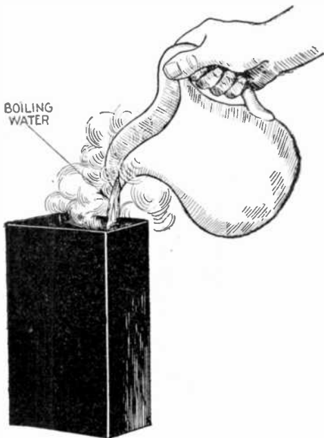
FIG. 1,797.— Battery repairs 25. Heat jar before placing it in the case. This may be accomplished by pouring boiling water in the jar. If hot water be not available play a light flame around the outside of the jar.
