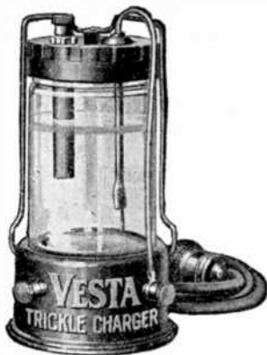
FIG. 1,886.—Vesta dry rectifier socket power "A" unit trickle charger. This unit is built in glass for clear visibility of all that is going on inside the unit and with the dry rectifier. This trickle charger operates through the medium of discs of two dissimilar metals, the elements being aluminum and copper sulphate. This construction gives contact at three points maintained under a central spring pressure to obtain efficient contact and eliminate heat. The low charging rate is .5 and the high rate 1\frac{1}{4} amperes. Uses the full wave for rectification. This unit, which included battery of either 4 or 6 volt sizes, has a built in visible hydrometer. An automatic relay is provided. This relay disconnects the charging current from the battery when set is turned on and if used with a B socket power unit not equipped with a relay, automatically connects the B when set is turned on.
