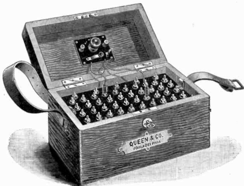
FIG. 1,505.—Queen portable silver chloride testing battery. The silver chloride cell has the advantage of long life, light weight, and compactness. The pressure of each cell when new is .8 volt.
