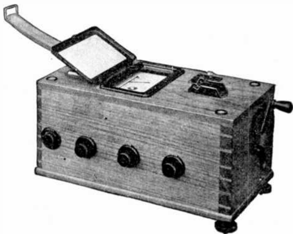
FIG. 1,575.—A high range "Megger" testing set ready for use.
