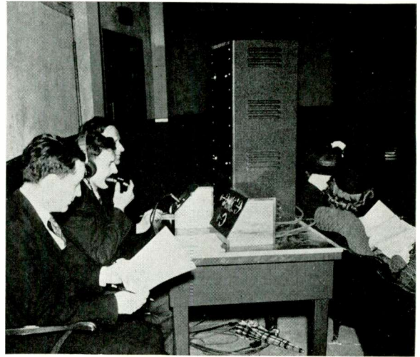
Fig. 5—Volume controls on 118A amplifiers are used as compensation controls for balancing purposes.
