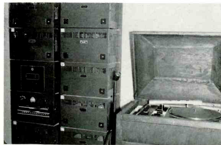
Below are shown amplifiers, control panels and reproducer panel at Ocean Beach Park, New London, and a view of the great boardwalk with central loudspeaker tower which floods a full half-mile of beach with beautiful music.
