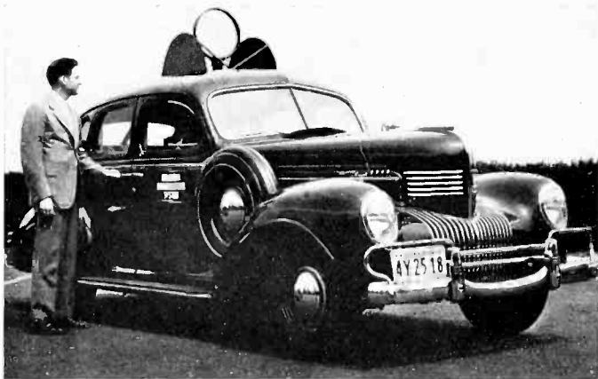
Columbia's new Field Intensity Measuring Car, which this year replaced one that had made more than 9,000 measurements in 53,000 miles of travel.
