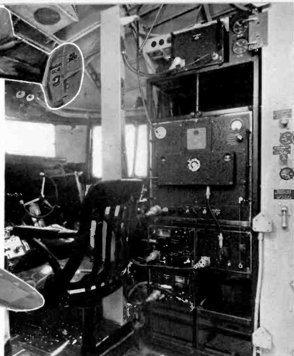
Western Electric radio equipment in the DC-4.
