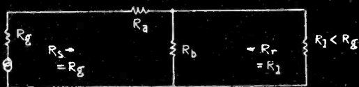
FIG. 7C UNSYMMETRICAL "T" NETWORK (FOR MATCHING UNEQUAL IMPEDANCES WITH MINIMUM LOSS) R_s = R_g AND R_r = R_1 < R_g WHEN R_a^2 = R_g^2 - R_g R_1 AND R_b^2 = R_g R_1^2 / (R_g - R_1)
